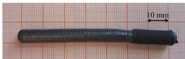
Fig. 1. Example of a BaTiO 3 -CoFe 2 O 4 composite boule grown via floating zone melting.
