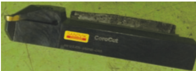
FIGURE 3: Tool of Sandvik Coromant carbide insert cutter with dimensions of 20 x 20 x 200 mm (w×h×l in mm).
