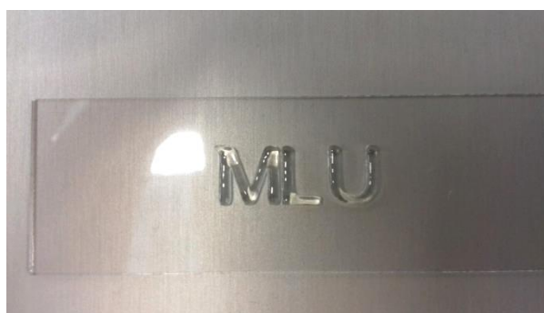
Figure 62. Supramolecular PIB-U2 was printed in an MLU shape with six layers.
