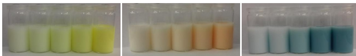
Figure 77. PLLA_MCT capsules with increasing amount of PF8BT (yellow), CN-PPV (orange) and PCPDTBT (blue).
