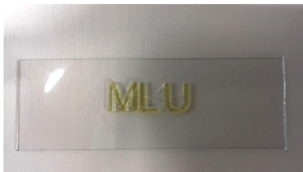
Figure 56: Supramolecular PIB-B2 was printed in an MLU shape with six layers.
