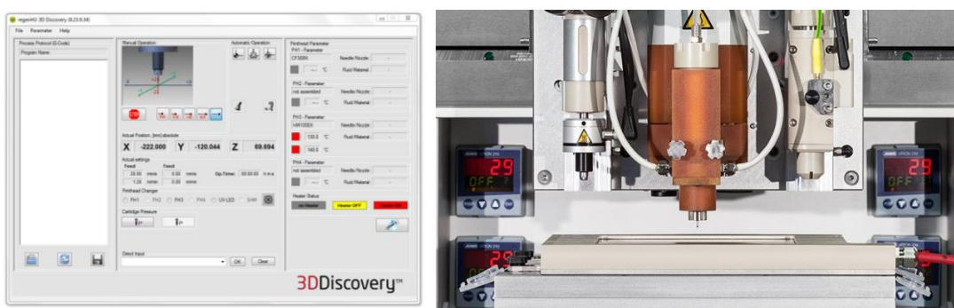
Figure 23. The human machine interface (HMI) for the regenHU 3D-Discovery , where most of the printing parameters could be changed (l.). The installed printing head of the 3D-printer are liquid inkjet head (drop-on-demand) and a polymer extruder with storage tank and screw extrusion unit (r.).
