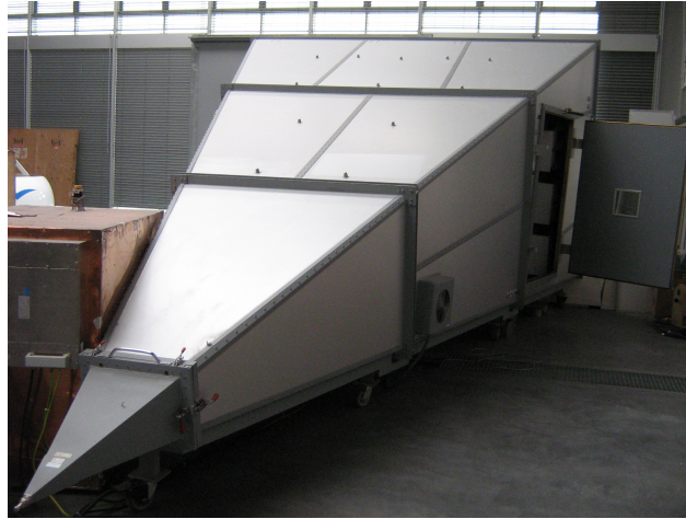
Figure 2.18: GTEM cell at the Otto von Guericke University in Magdeburg
