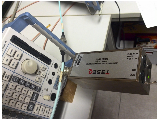
(a) measurement of the output power of the comb generator
