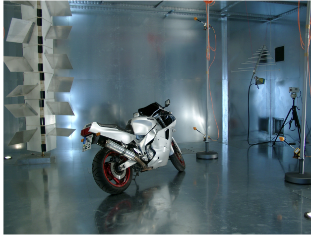
Figure 2.19: Mode stirred chamber (MSC with dimensions of 7.9 m \times 6.5 m \times 3.45 m) with a lowest usable frequency (LUF) of 200 MHz at the Otto von Guericke University in Magdeburg. Copyright © Chair of Electromagnetic Compatibility, University of Magdeburg, Germany
