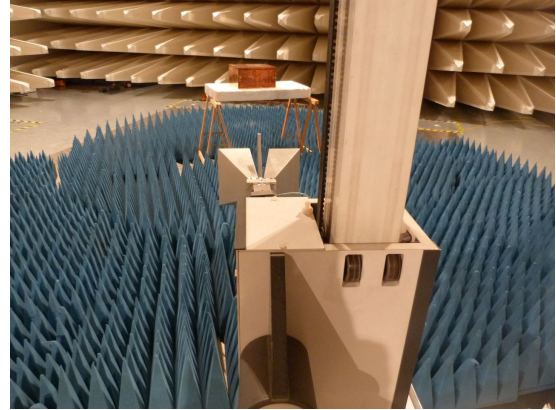
(b) SAC with floor absorbers to realize the fully anechoic effect at the Otto von Guericke university in Magdeburg with the receiving antenna at a distance of 3 m from the EUT and at the height of 1 m
