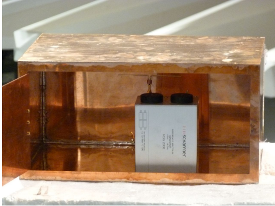
(a) The enclosure with the front plate held by two conducting straps (right strap not shown because of the opened front plate) as the EUT, with a small antenna mounted on the comb generator acting as a source inside the box
