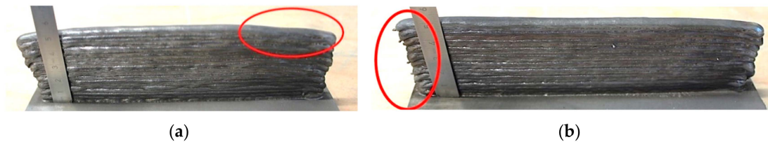
Figure 2. Influence of a front-feeding (a) or rear-feeding (b) cold wire on the specimen geometry.
