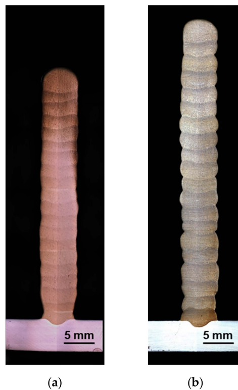
Figure 4. Geometry of specimens consisting of 20 layers each, (a) without cold wire, (b) with 23.1% cold wire percentage.
