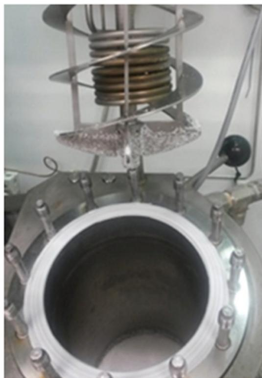
**Figure 9.** 5 L bulk-gas-phase reactor with power compensation heater and double helical ribbon stirrer.
