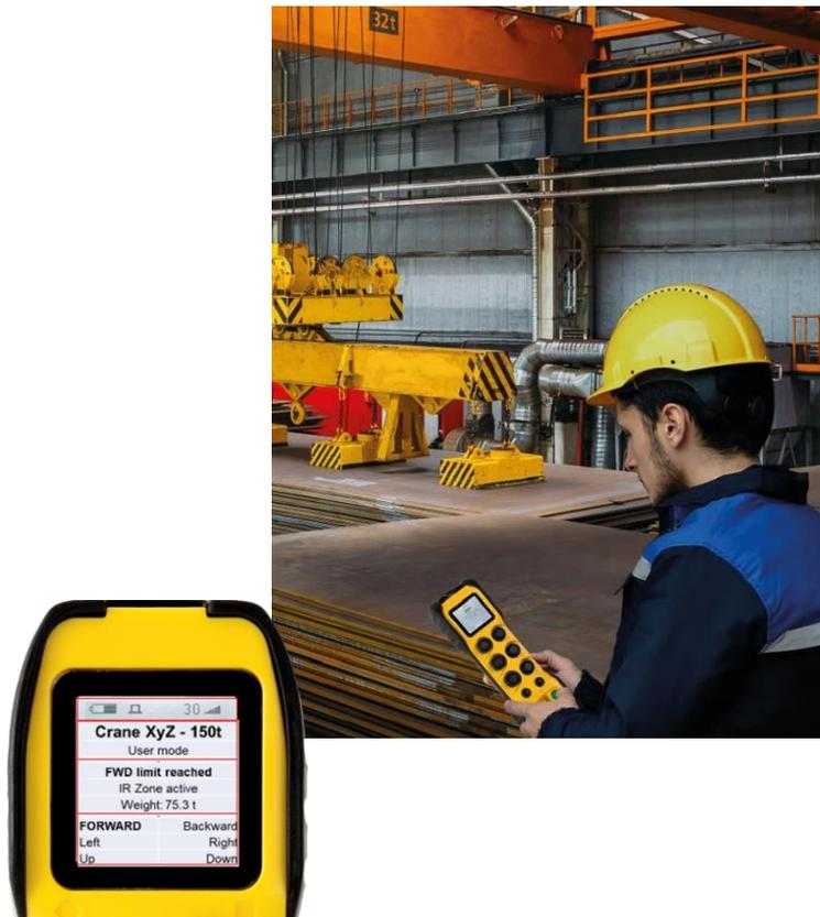
Figure 3: Crane operator using a screen based remote control
