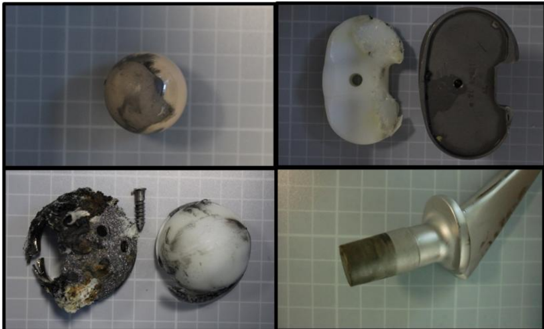
Figure 2: Representative photographs of retrieved TJA, top left: signs of wear in a ball head of a THA; top right: signs of wear and destruction of the inlay in a tibial part of a TKA; bottom left: fracture of the acetabular component of a THA; bottom right: corrosion of the taper of a THA
