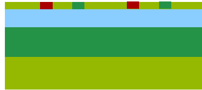
3) TiN etching and island etching
