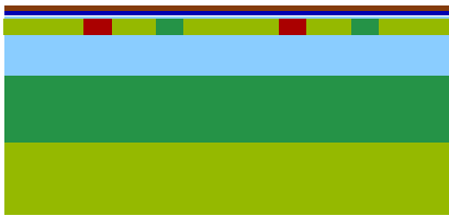
2) Interfaceoxide growth and HfZrO2/TiN deposition
