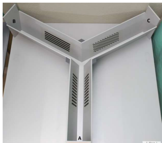
Figure 10. Y-maze set up. The three arms of the y-maze are marked with different patterns, allowing the mice to orientate.
