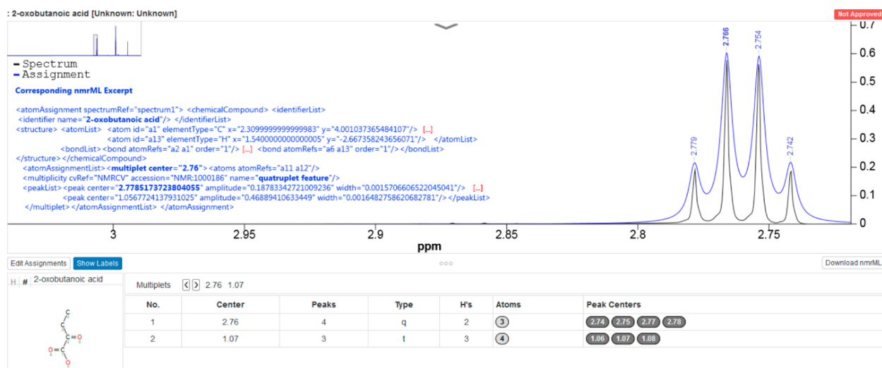
Figure 2. Assignment of an identified molecule in a single compound spectrum, generated in nmrML-Assign and displayed using the JSpectraViewer (JSV). An uploaded raw FID for the 2-oxobutanoic acid reference compound was automatically processed with Bayesil. The resulting interactive JSV spectrum then allows the assignment of peaks to specific atoms, using the nmrML-Assign tool. The assignment metadata is then saved in the nmrML format (see https://github.com/nmrML/nmrML/tree/master/examples/reference_spectra_examples/hmdb ). An excerpt view of the corresponding nmrML code (blue code inset) is shown for the quadruplet assignment (Multiplet no. 1) of the second peak (bold code). The corresponding HMDB entry is available from http://www.hmdb.ca/metabolites/HMDB000005 , with the ^1\text{H} spectrum found at http://www.hmdb.ca/spectra/nmr_one_d/1024 .
