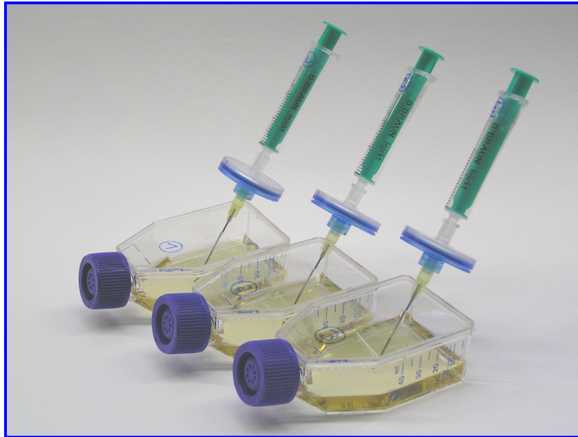
Fig. 8 A set of three dynamic in vitro models, containing a 70 mL canted neck cell culture flask filled with 20 mL broth containing a defined bacterial inoculum, a cannula firmly inserted in the flask wall, a membrane filter unit, and a 2 mL syringe; respectively. For a more detailed description see text.
