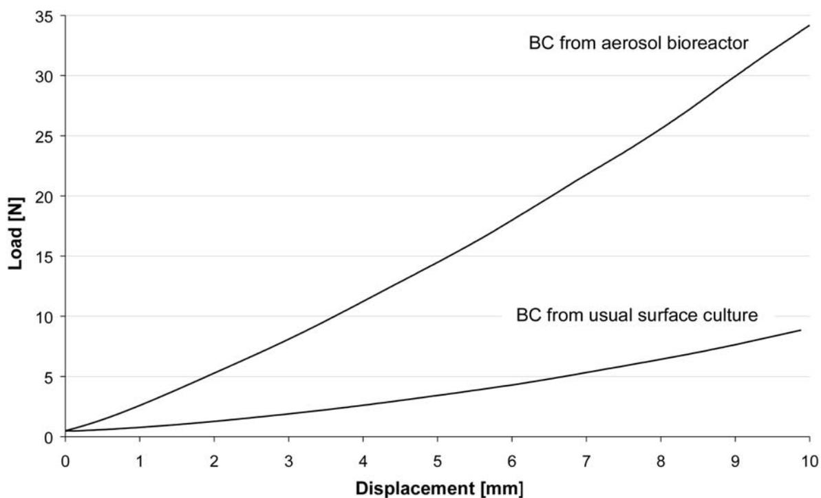
**Figure 6.** Load-displacement curves of BC from aerosol bioreactor and BC from static surface culture
