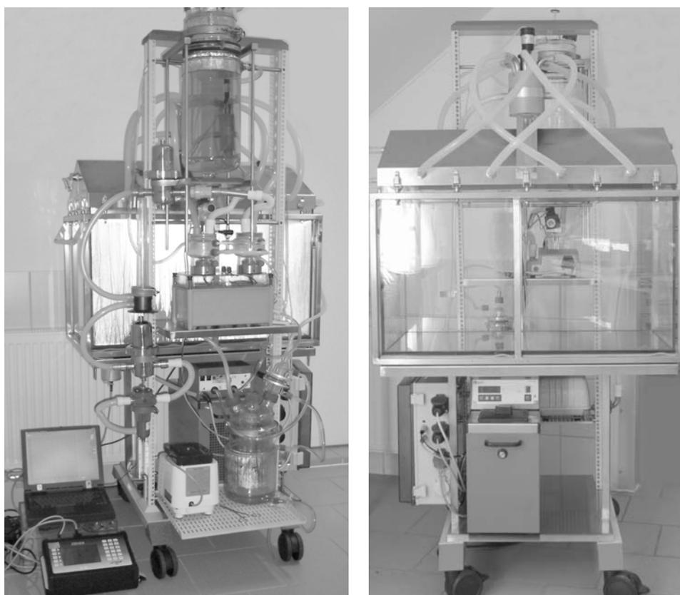
**Figure 3.** The aerosol bioreactor (left hand: back; right hand: front)
