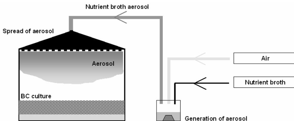
**Figure 2.** Direct supply of substrate by an aerosol
