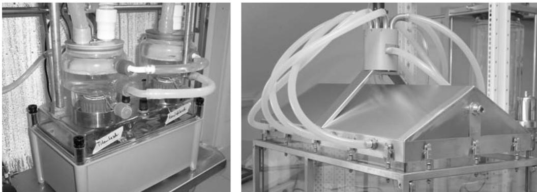
**Figure 4.** The substrate aerosol generator (left) and aerosol spreading (right)
