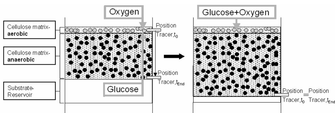
**Figure 1.** Changing from an indirect to a direct feeding of both substrates (glucose and oxygen)
