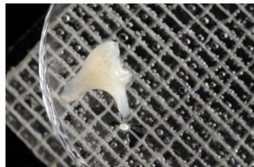
Abb. 7: Amboss, eingebettet in PMMA
