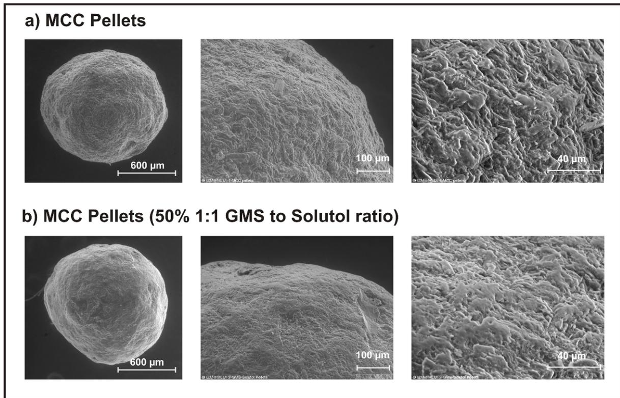
**Figure 5.2** ESEM Pictures of the control MCC pellets and the self-emulsifying pellets.
