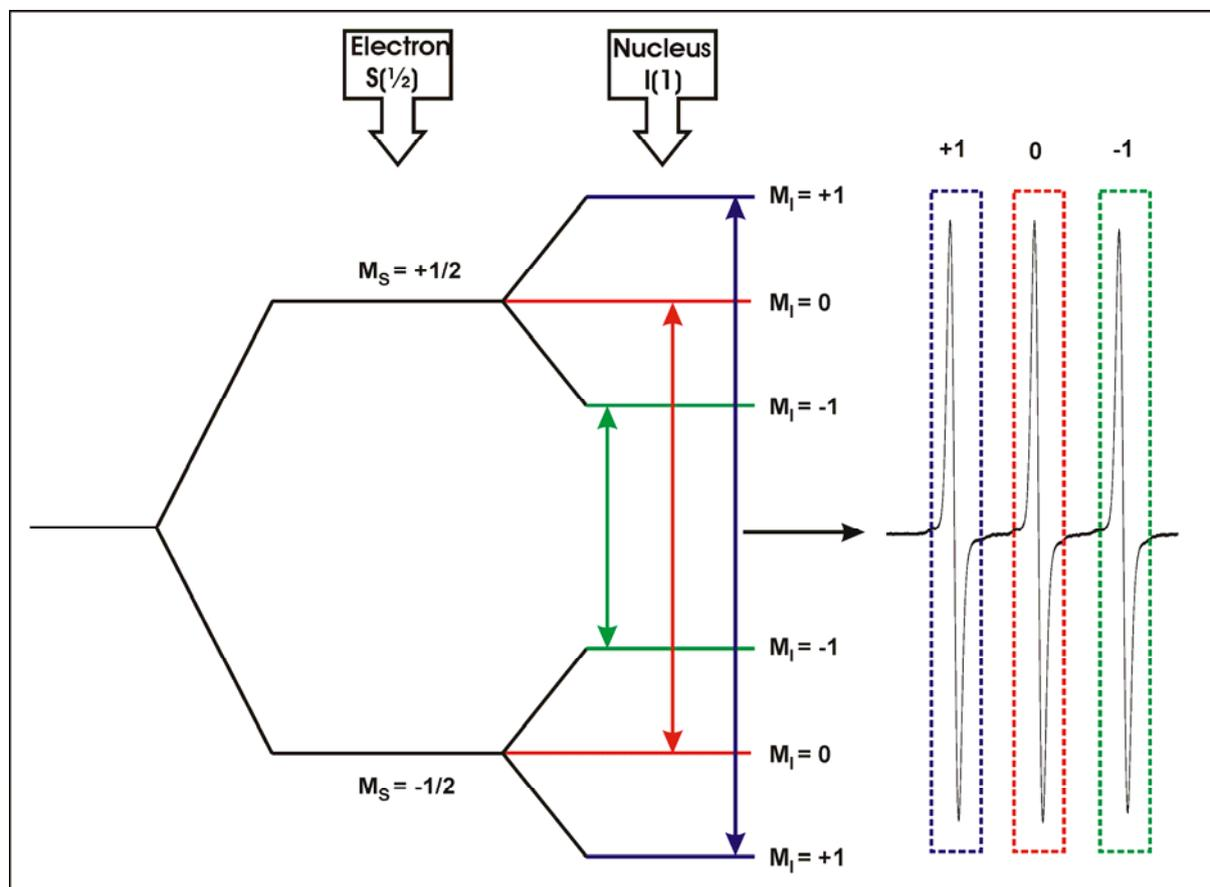
**Figure 8.1** Energy levels and transitions for a nitroxide spin probe ( $^{14}\text{N}$ ) with electron spin ( $S = 1/2$ ) and nuclear spin ( $I = 1$ ) (adapted from Ref. [176]).
