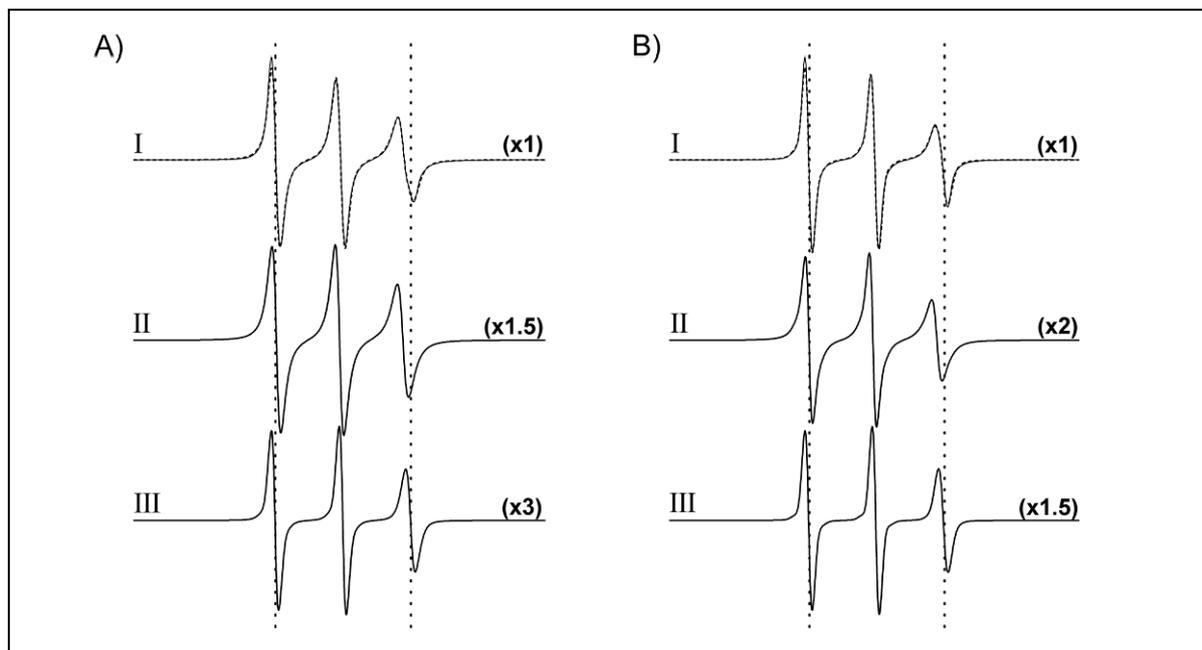
**Figure 12.3** ESR simulation spectra of TB after A) 0 min, and B) 30 min of the digestion of 1% (w/v) of The SE mixture B5 in the digestion buffer under FaSSIF conditions. I) Experimental spectrum (bold line) and simulated spectrum (dotted line), II) spectrum of the lipophilic species, III) spectrum of the hydrophilic species.
