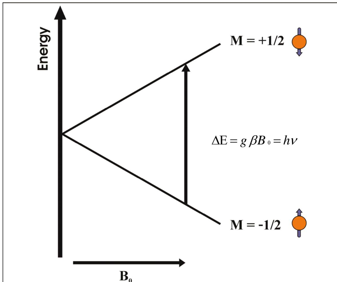
**Figure 7.1** Energy level diagram showing the two possible states of an electron ( $S = \frac{1}{2}$ ) in an applied magnetic field, The lower energy level corresponds to the electron spin being parallel to the direction of the magnetic field, while its orientation is reversed in the upper energy level, as indicated by the arrows on the right side (modified from Ref. [169]).
