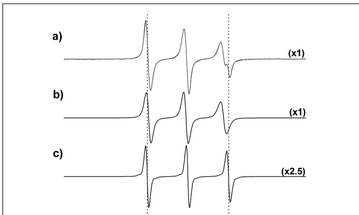
**Figure 7.3** ESR simulation spectrum of TB in the emulsion resulted from the dispersion of SE mixture B5 in phosphate buffer. a) Experimental spectrum (bold line) and simulated spectrum (dotted line), b) spectrum of the lipophilic species c) hydrophilic species.
