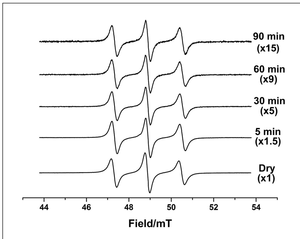
**Figure 20.3** ESR spectra of TB loaded pellets before, 5, 30, 60 and 90 min after buffer exposure in the flow cell system.
