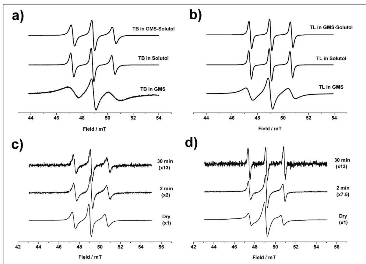
**Figure 7.2** ESR spectra of TB (a) and TL (b) loaded formulation ingredients and mixtures. ESR spectra of TB (c) and TL (d) loaded pellets before, 2 and 30 min after buffer exposure in the flow cell system.
