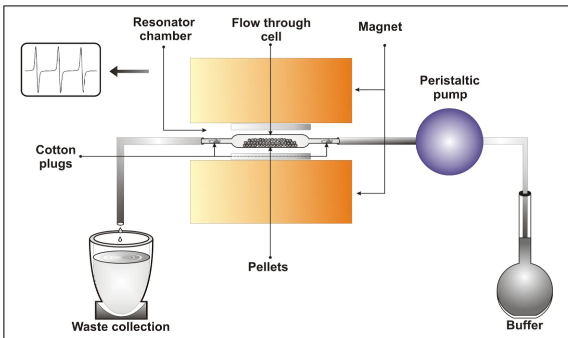
**Figure 3.2.** Schematic diagram showing the setup of the ESR flow through system. A flow through cell is placed inside the measurement (resonator) chamber between the magnets. The cell is connected from one end to a peristaltic pump and the other end to the waste collection.
