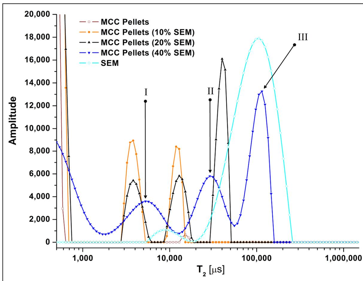
**Figure 18.3** NMR  $T_2$  distribution of MCC ( $\blacksquare$ ), SE mixture B5 ( $\blacklozenge$ ), and pellets with 10 ( $\bullet$ ), 20 ( $\blacktriangle$ ) and 40% ( $\blacktriangledown$ ) of incorporated SE mixture B5.
