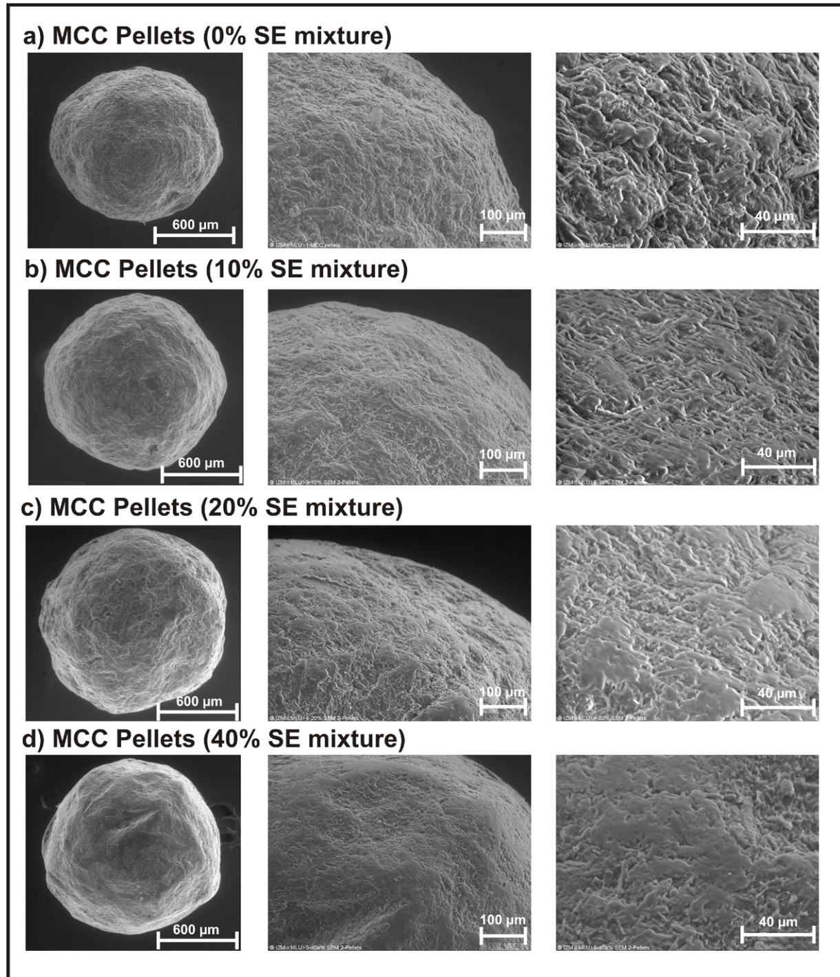
**Figure 15.3** ESEM Pictures of self-emulsifying pellets with different load of the liquid self-emulsifying lipid mixture.
