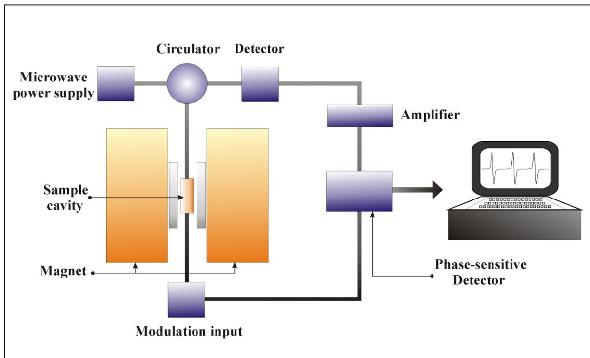
**Figure 9.1** Schematic presentation of the main components of an ESR spectrometer.
