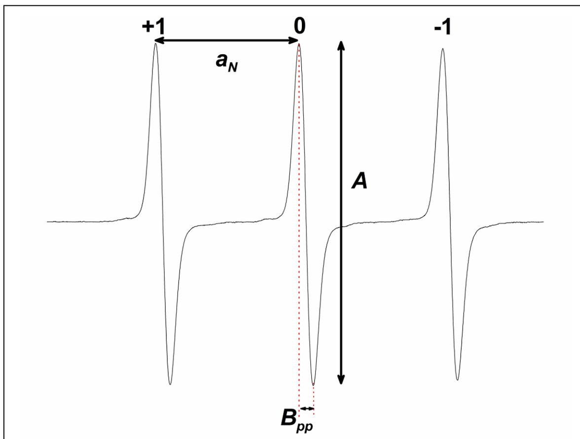
**Figure 10.1** A typical nitroxide spectrum showing the important spectral parameters.  $B_{pp}$  is the peak to peak line width,  $a_N$  is the hfs constant, and  $A$  is the peak amplitude.
