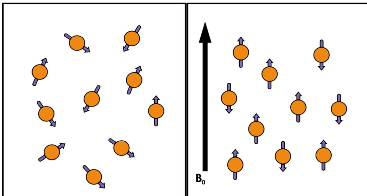
**Figure 6.1** A schematic diagram illustrating the Zeeman effect. Left, random orientation of the electron spins. Right, alignment of the electron spins with or against the external magnetic field  $B_0$  (modified from Ref. [169]).
