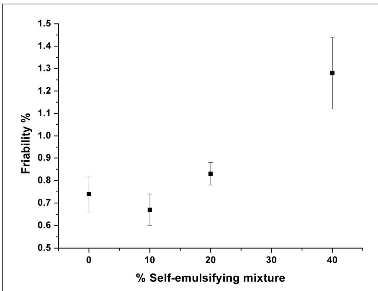
**Figure 16.3** Friability % (mean  $\pm$  SD, n=3) of MCC pellets prepared with different % of self-emulsifying mixture incorporation.
