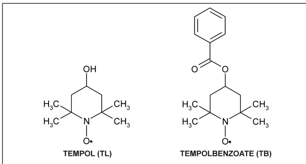
**Figure 2.2** Chemical structures of the ESR spin probes Tempol and Tempolbenzoate.
