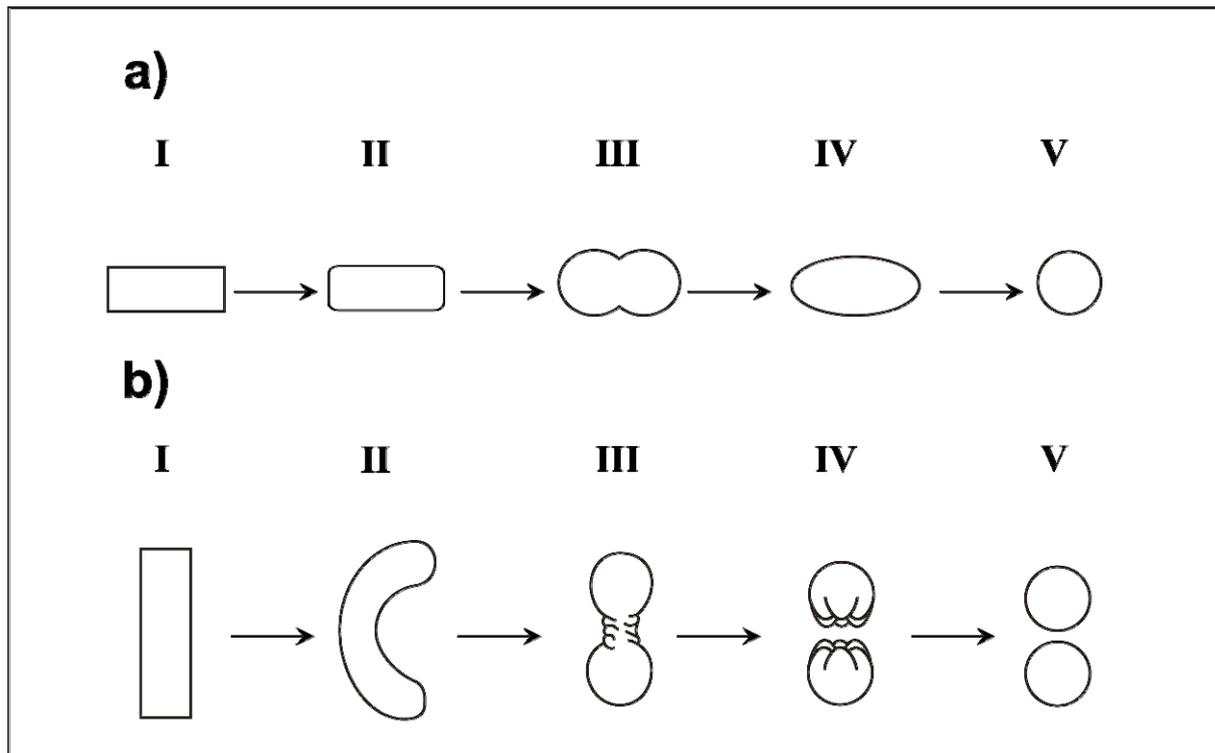
**Figure 4.1** Pellets formation mechanism according to a) Rowe [152]- I. Cylinder, II. Cylinder with rounded edges, III. Dumb-bell; IV, Ellipse, V Sphere. (b) Baert et al [158]- I. Cylinder, II. Rope, III. Dumb-bell, IV. Sphere with a cavity outside, V. Sphere. (from reference [165]).
