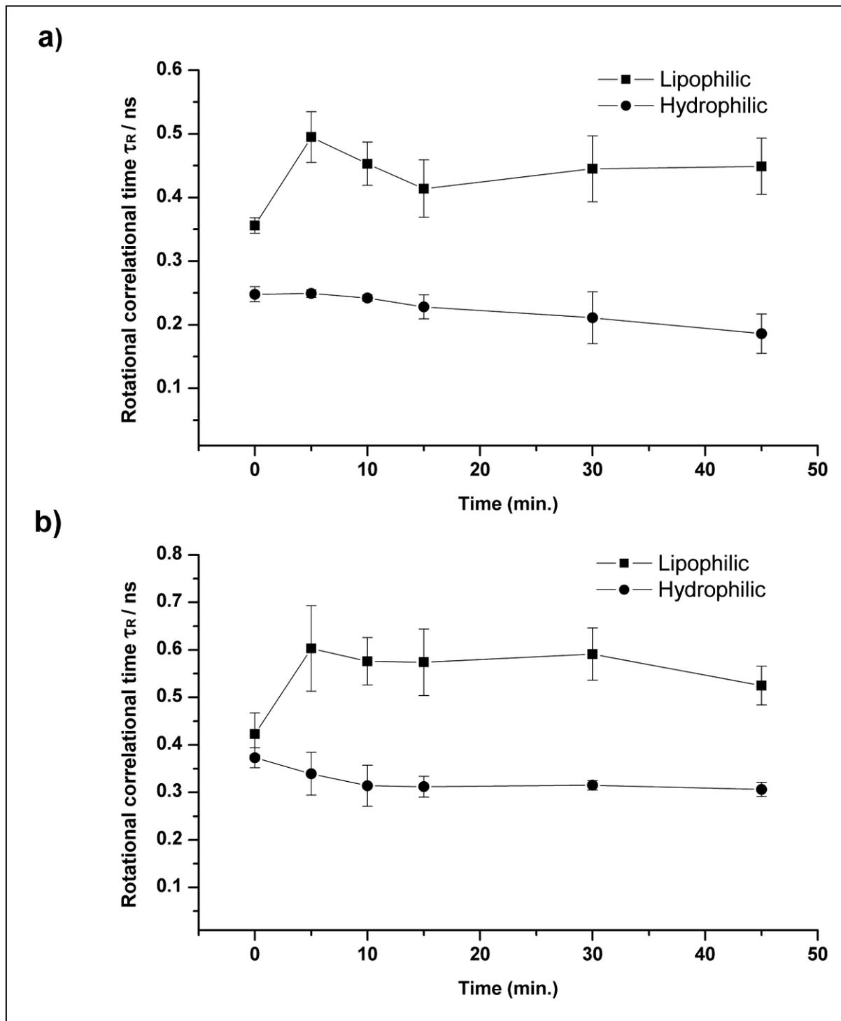
**Figure 14.3** Change of rotational correlation time, for lipophilic and hydrophilic species, as a function of time after the digestion of 1% (w/v) of the SE mixture B5 in the digestion buffer under a) FaSSIF and b) FeSSIF conditions.
