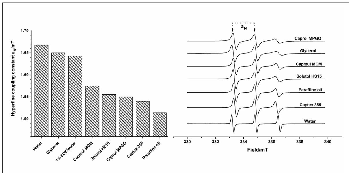
**Figure 4.3** ESR spectra of TB in environments with different polarity and viscosity. The hyperfine coupling constant  $a_N$  is sensitive to the polarity of the environment (left diagram) which is used to monitor the partitioning of spin probes between compartments with different polarity. Please note the effect of increasing the viscosity on the broadening of the line width (right diagram).
