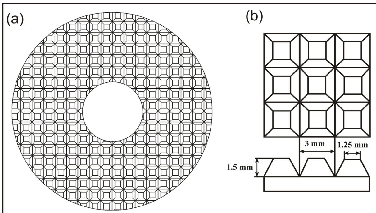
**Figure 3.1** Schematic presentation of the frictional plate used in the radial plate spheronizer showing (a) typical grid pattern (the cross hatched design), and (b) details of grid pattern and a cut away view of the plate with the dimensions of plate design.
