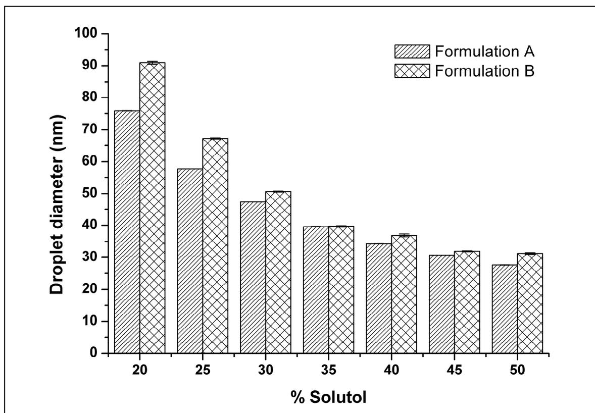
**Figure 3.3** Effect of Solutol content on the droplet diameter (mean  $\pm$  SD,  $n=3$ ) of the emulsions produced by dispersing SE mixtures in water.
