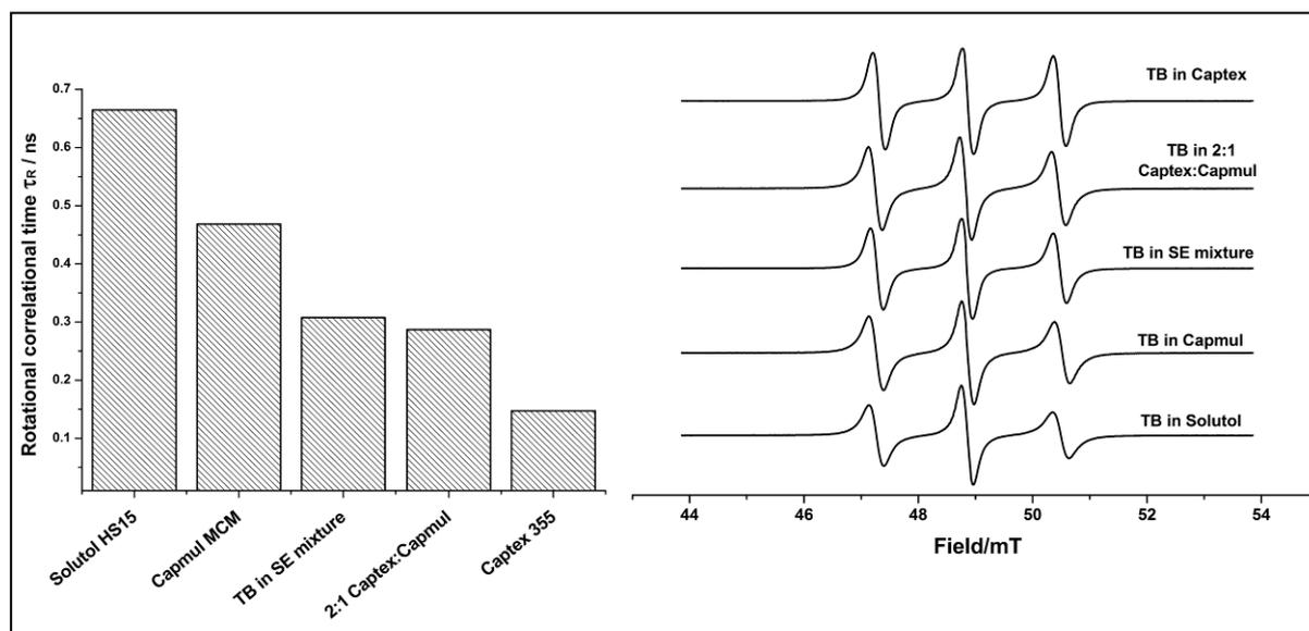
**Figure 19.3** ESR spectra of TB in different formulation components and mixtures, reflecting the sensitivity of the line shape (right) and rotational correlation time (left) to the viscosity of different media.
