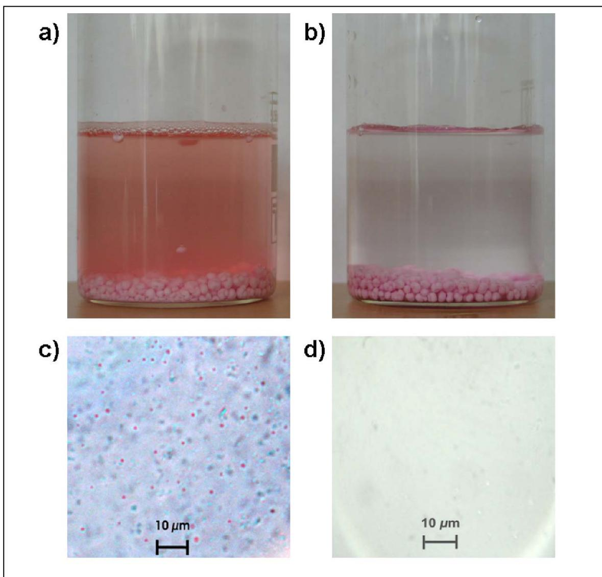
**Figure 6.2** Photograph showing the release media of (a) self-emulsifying pellet formulation. (b) Reference pellets, containing Sudan red dye, after 30 min of dissolution in distilled water at a temperature of 37 °C. And microscopic picture of the release media of (c) self-emulsifying pellets (d) reference pellets.
