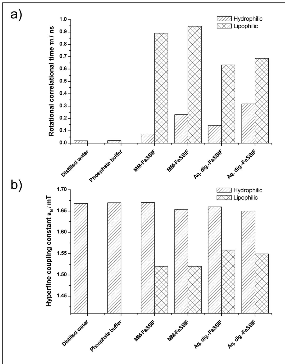
**Figure 11.3** Values of a) Rotational correlation time and, b) Hyperfine coupling constant, for TB in different control media.
