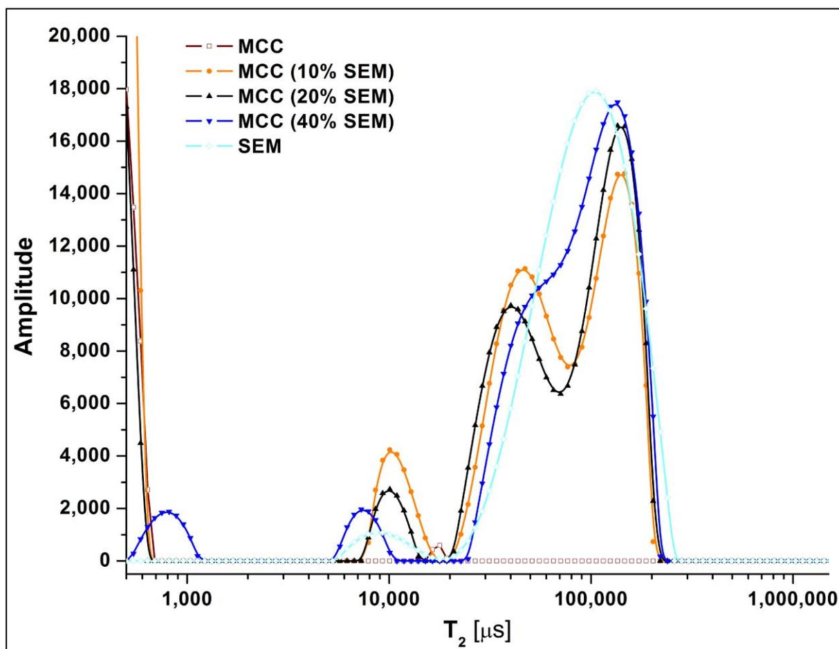
**Figure 17.3** NMR  $T_2$  distribution of MCC ( $\square$ ), SE mixture B5 ( $\diamond$ ), and physical mixtures of MCC with 10 ( $\bullet$ ), 20 ( $\blacktriangle$ ) and 40% ( $\blacktriangledown$ ) SE mixture B5.
