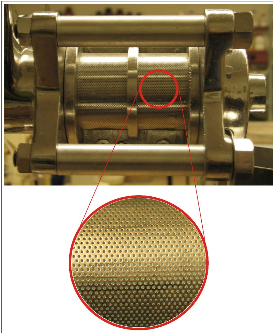
**Figure 2.1** Photograph of the twin screw radial discharge extruder.
