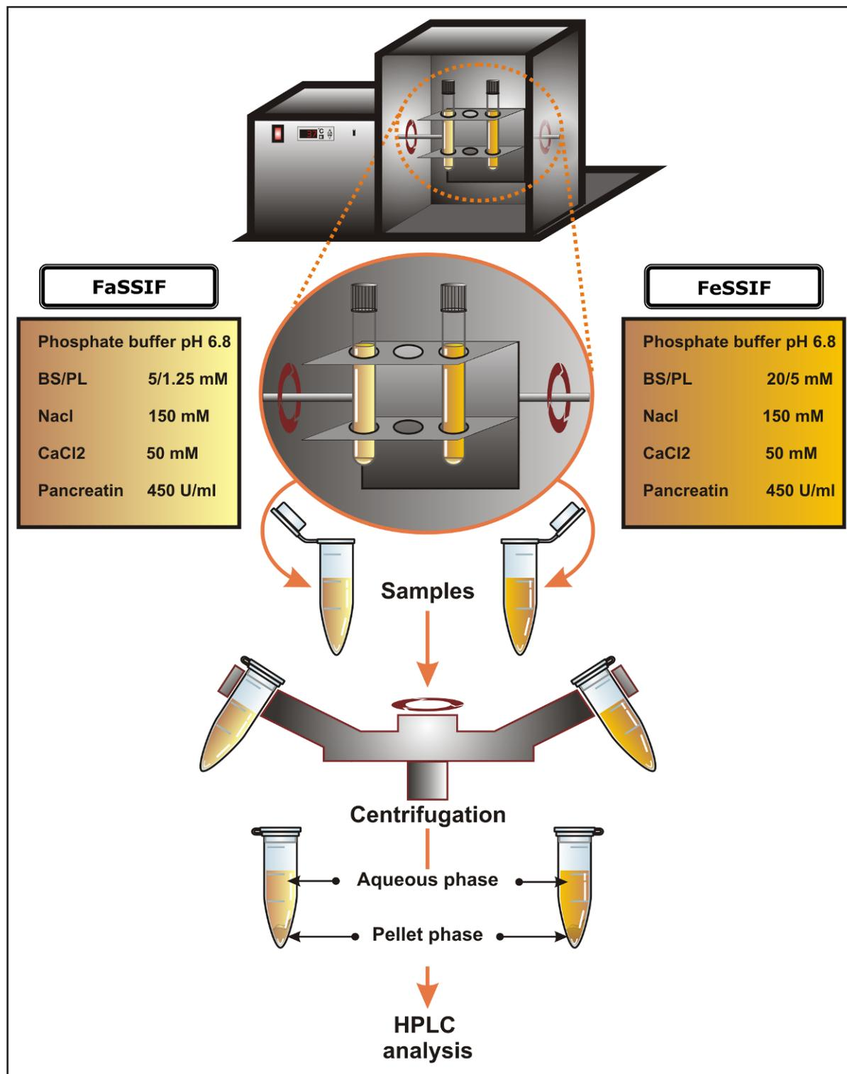
Figure 2.3 schematic presentation of the in vitro digestion experiment
