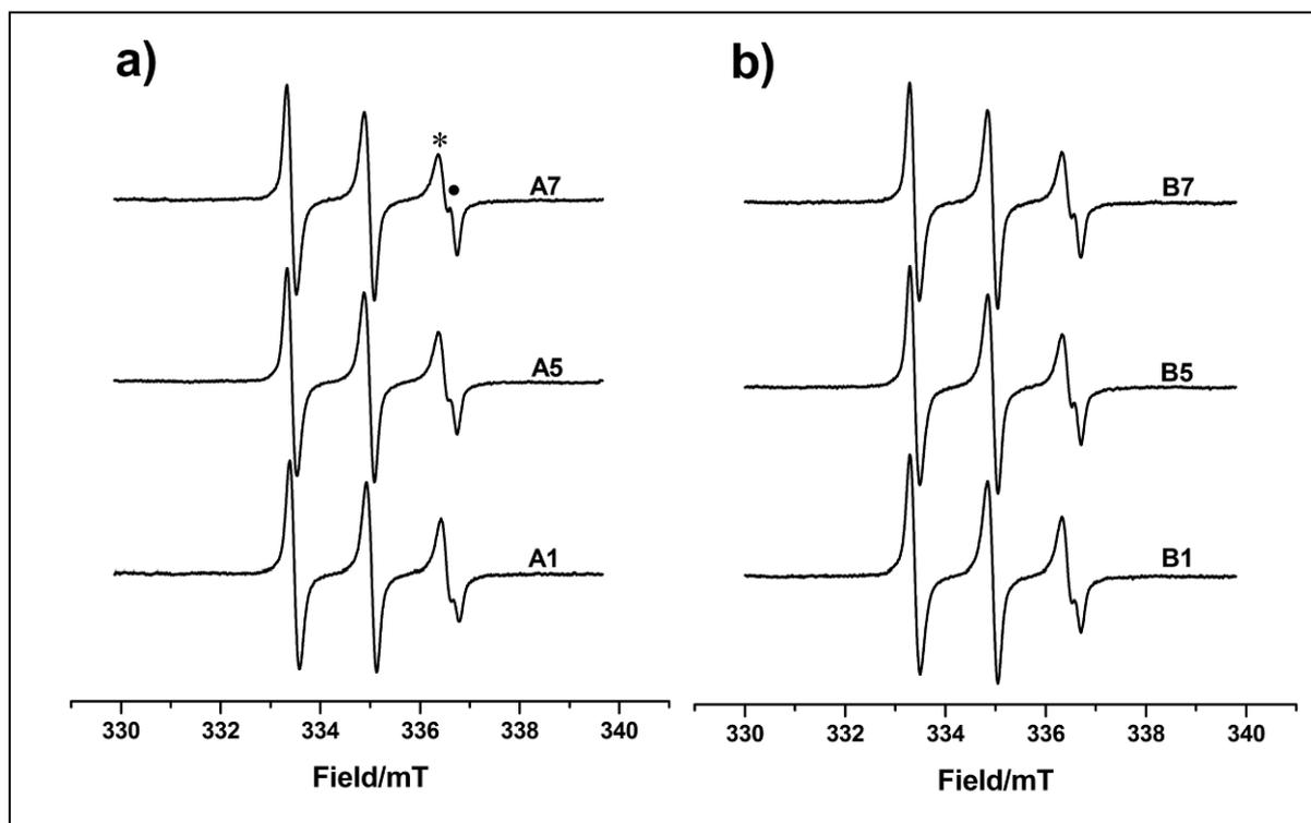
**Figure 6.3** ESR spectra of TB in the emulsion resulted from the dispersion of SE mixtures a) from formulation A b) from formulation B in phosphate buffer pH 6.8. (\* refers to the lipophilic while • refers to the hydrophilic species).
