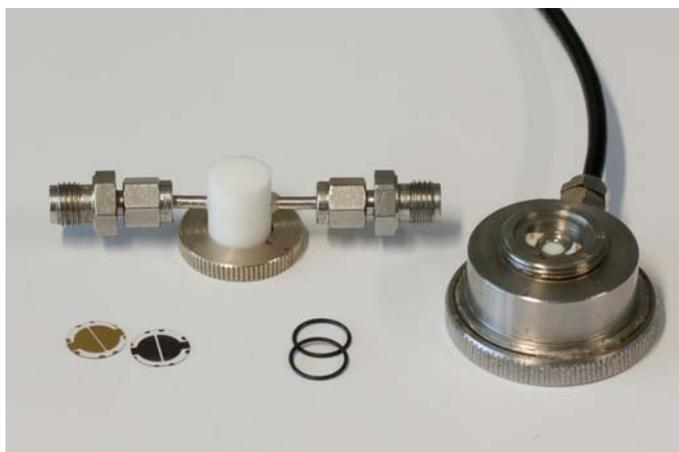
Figure 7-1: VOC measurement cell for LFE sensor.
