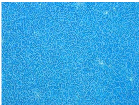
Figure 5-5: Typical image of homogeneously distributed NP film on silicon substrate ( $\times 20$  times).
