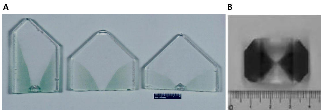
Fig. 6.16: Face-specific incorporation of \text{Cr}^{3+} (A) [Zai99] and a dye (B) [Hir02] into the crystal lattice of potassium dihydrogen phosphate
