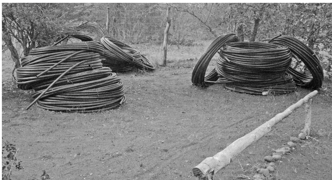
Figure 89 – The plastic pipes for water supply at the entrance of the Covane Lodge (photograph by the author, September 8, 2006).
