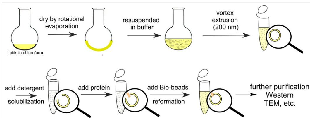
**Figure 2.11: Scheme for the reconstitution using the detergent-mediated method**
