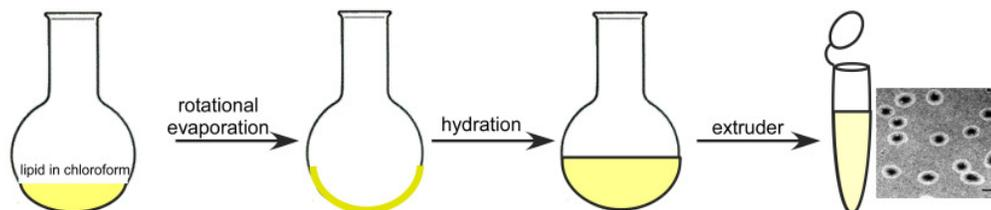
**Figure 2.5. Schematic representation of the standard protocol for liposome preparation.** As an example, the TEM image of prepared PC liposomes was shown on the right (scale bar: 200 nm).
