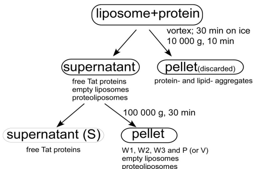
**Figure 2.7: Schema for the purification of proteoliposomes by the centrifugation.**
