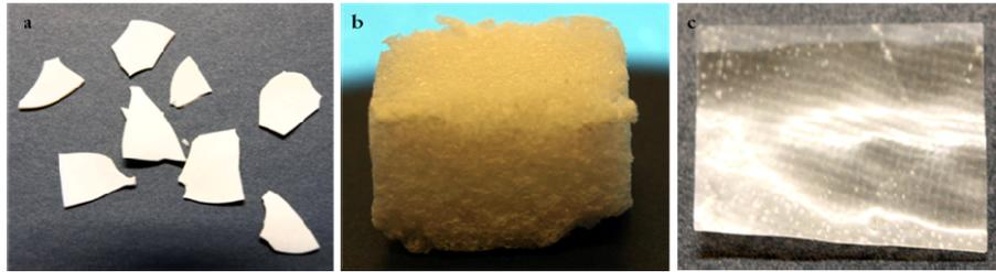
**Figure 81: Implants from PHB/HA composites for tissue engineering applications a) compact structures, b) porous 3-D structures and c) Sandwich structure of membrane and electrospun ma**
