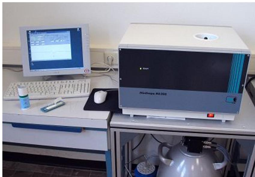
Fig. 2.3-1: The ESR spectrometer Miniscope MS 200 (X-Band).
