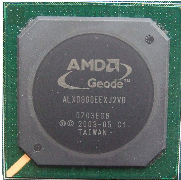
Figure 2.2: AMD Geode is an x86 compatible system-on-a-chip.
