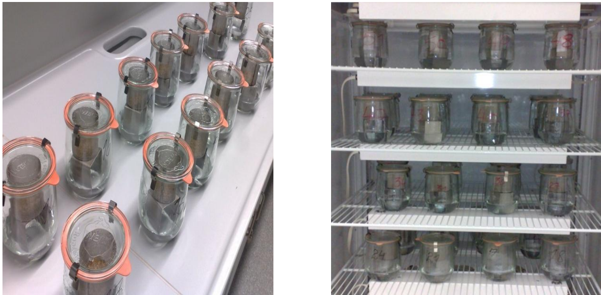
Figure 5: (a) Steel cages containing seeds placed on steel stands above 200 ml distilled water and sealed in glass jars and (b) Glass jars are placed in a climatic chamber at 43°C for 72 hours
