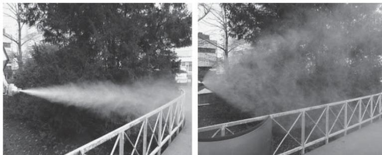
**Fig. 11.** Standard spray jet (left) and wide spread spray jet (right).
