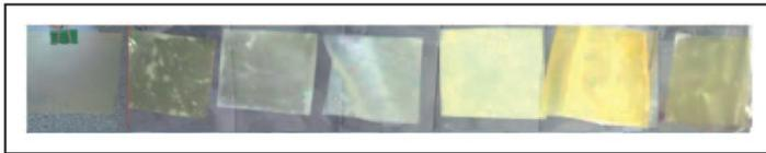
**Figure 9.** Collagen film after treatment with different test fluids for 1 h (from left to right: control film [without treatment], oil-mix, fuel-mix, screen wash fluid, deionized water, sodium hydroxide [NaOH; 1%], sulfuric acid [H<sub>2</sub>SO<sub>4</sub>; 1%]).
