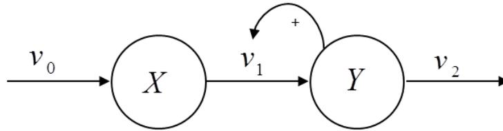
Figure 1.1: Network diagram of Higgins-Sel'kov oscillator. The supply rate of the substrate, X, is  $v_0$ , the conversion of substrate to product Y occurs at a rate of  $v_1$  and product Y is consumed at a rate of  $v_2$ .
