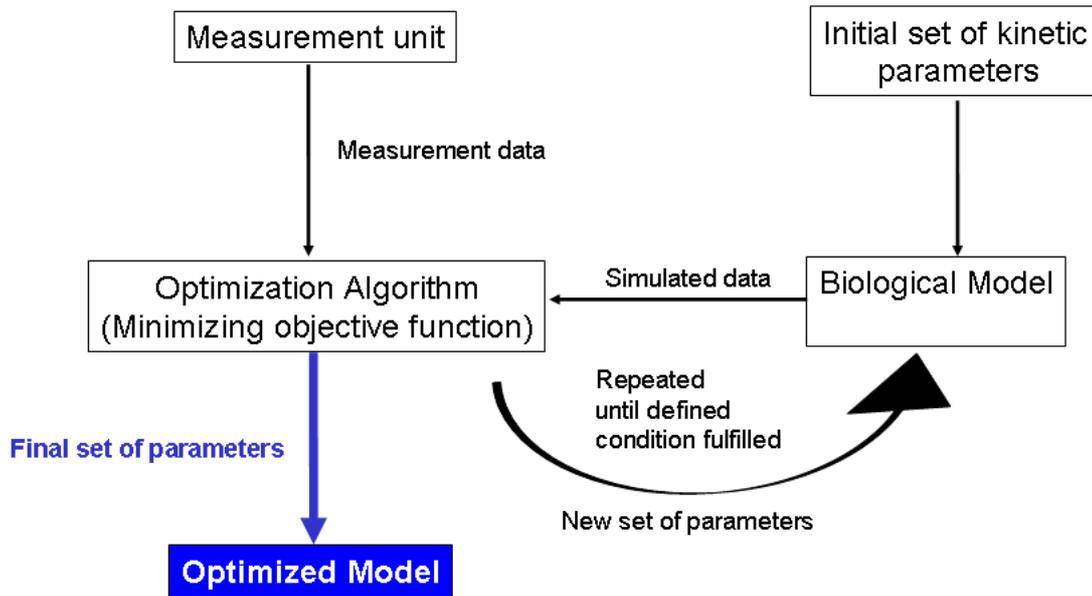
Figure 1.4: General scheme of the optimization method. Simulated data comes from the model, and measurement data comes from the measurement unit. The optimization is repeated until a pre-defined condition is met.
