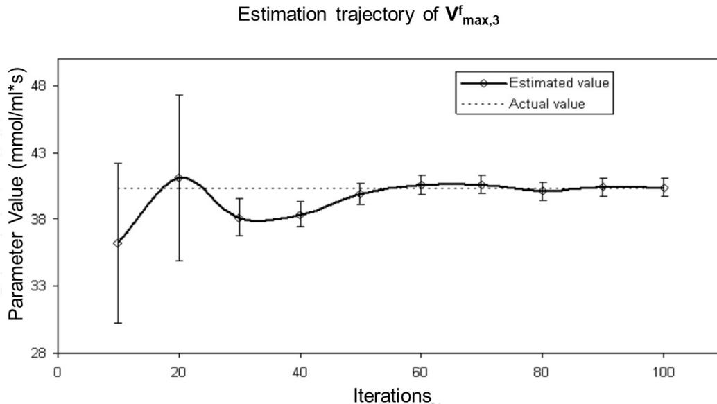
Figure 3.3: Estimation trajectory of  $V_{\max,3}^f$  from a representative sample run (run 5) with standard deviation. The dashed line represents the actual value and the solid line represents the estimation trajectory. The vertical bar represents the standard deviation. For visibility and ease in analysis plotting begins with the 10<sup>th</sup> sampling point and the standard deviation is given for every 10<sup>th</sup> sampling point.
