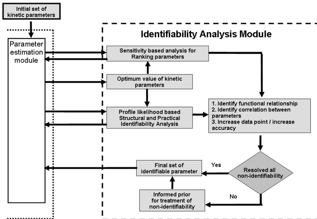
Figure 2.2: Identifiability analysis module. This module conducts the identifiability analysis of the parameters, including the ranking and identifies the correlation and the non-linear functional relationship between the parameters. The initial set of parameter values used in this module comes from the CSUKF in the parameter estimation module.
