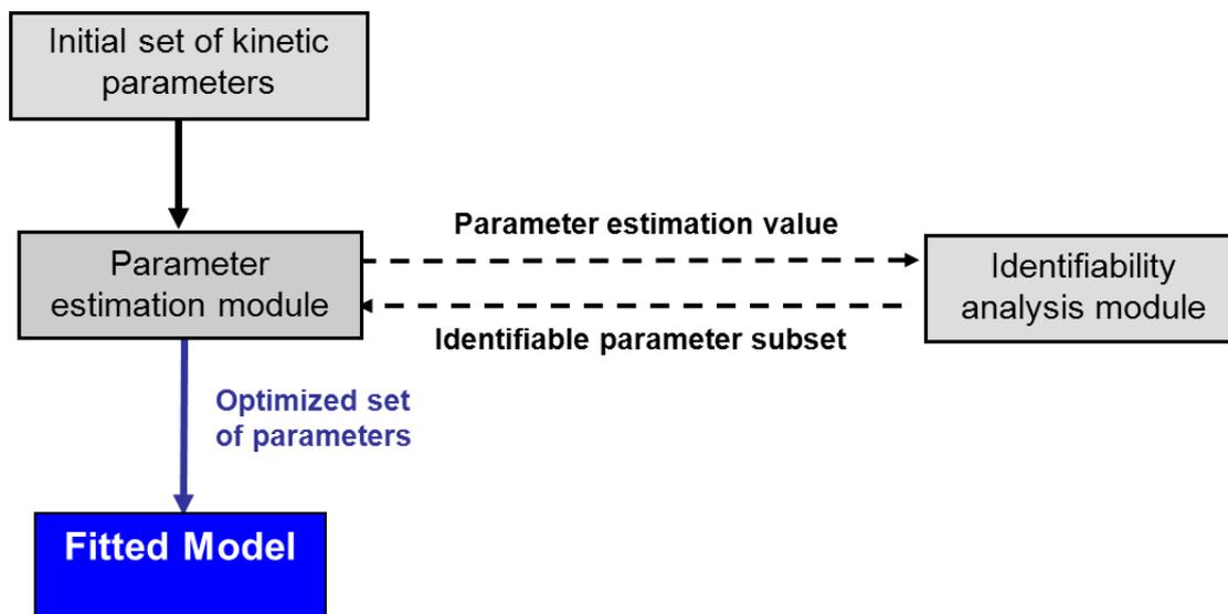
Figure 2.1: Complete parameter estimation framework. For different calculations the identifiability analysis module uses the optimized data of the parameter estimation module.
