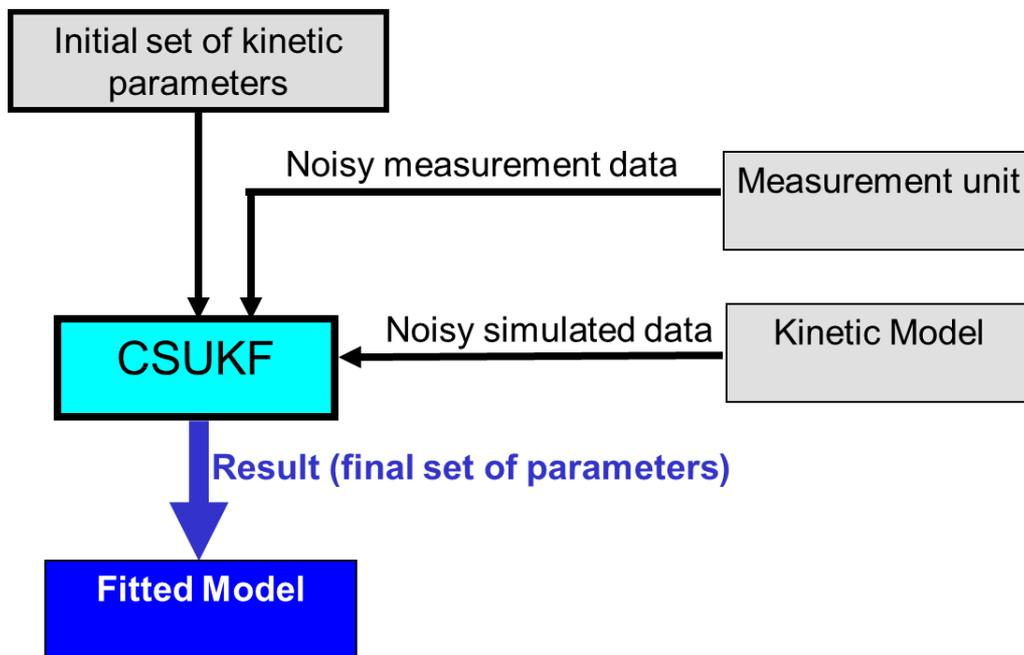
Figure 2.3: Parameter estimation module. CSUKF iteratively estimates parameter values by minimizing the difference between the noisy simulated data and the noisy measurement data
