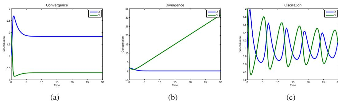
Figure 1.2: Dynamic behaviour of Higgins-Sel'kov oscillator. The value of the parameters are  $k_1 = k_2 = 1.1$ , and different values of parameter  $k_3$ . a) Converging, with  $k_3 = 0.6$ , b) diverging with  $k_3 = 1.6$  and, c) oscillating with  $k_3 = 1.1$ .
