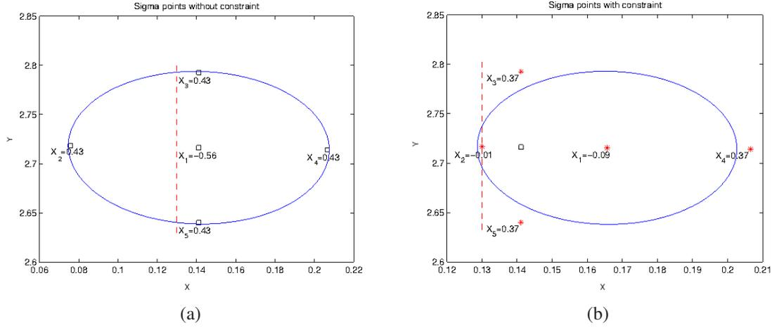
Figure 2.5: Selection of sigma points in the presence of constrain boundary. The dashed line represents the boundary. It shows how the sigma points are projected onto the boundary in case they violate it. The number on each of the sigma points represent their corresponding weights
