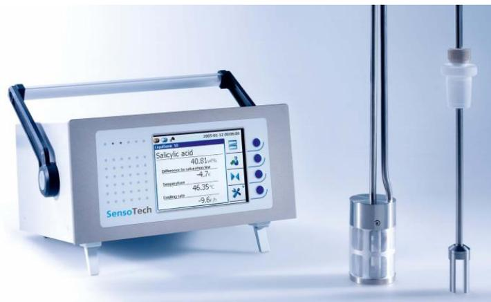
**Fig. 14-1:** OCM device with controller, protected and unprotected ultrasound sensor [Sen13].
