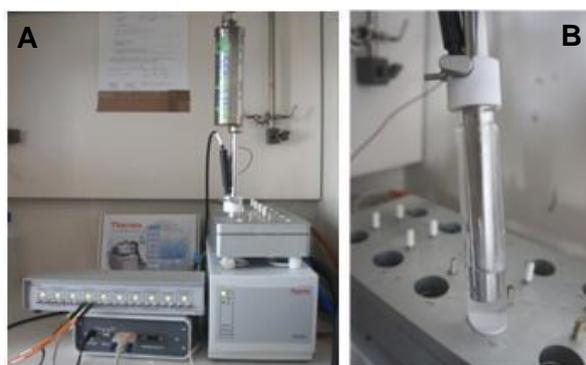
**Fig. 14-6:** Experimental setup of the ORM performed in the STEM Integrity 10 reaction station (A) and enlarged view on the ORM sensor integration in the reaction vessel (B).
