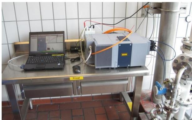
**Fig. 14-4:** Bruker Matrix-F process spectrometer in the pilot plant.
