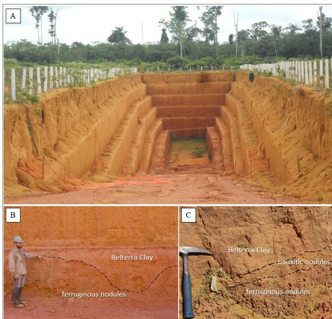
Figure 24 Belterra Clay exposed in Rondon do Pará with the general view of the Círiaco pilot-mine sampling site (A), showing the abrupt contact of the Belterra Clay with ferruginous nodules (B) and with bauxitic nodules (C).
