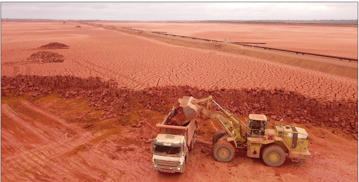
Figure 11 Bauxite washing clay in the tailing pond located in the facilities of the bauxite mine of Mineração Paragominas SA (Hydro), in Paragominas, Brazil. The material in the photo is dried and being removed. Source: Hydro Paragominas.
