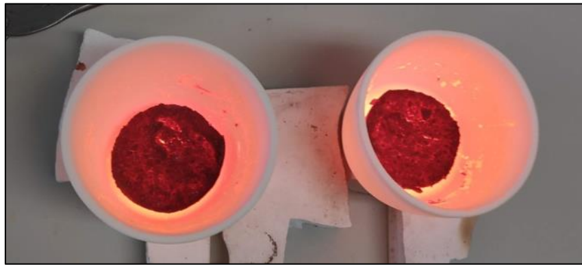
Figure 22 Clinkers in alumina crucibles during the cooling process after firing at 1250 °C for 1 hour.
