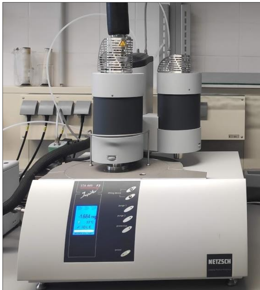
Figure 18 Netzsch STA 449 F3 Jupiter thermo-analyser.
