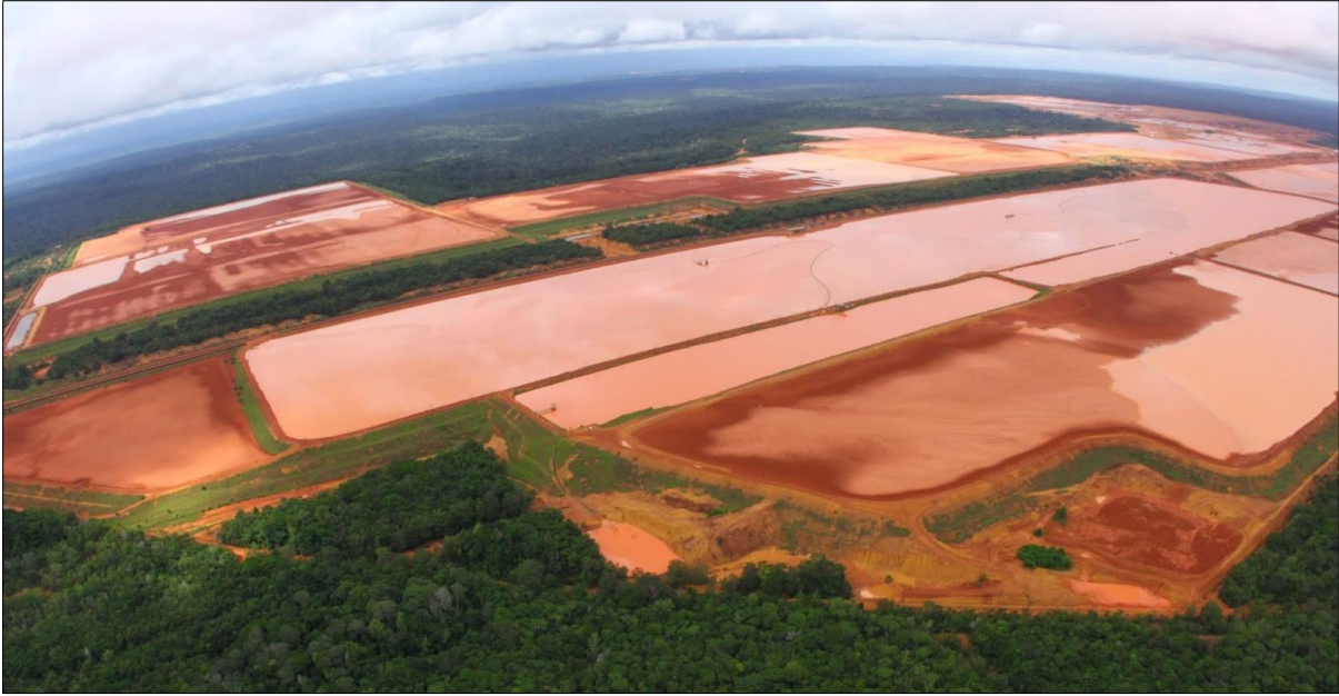
Figure 10 Tailing ponds with bauxite washing clay residue in Porto Trombetas, Lower Amazon, Brazil. Photo from Carlos Penteadó, Documentária Fotographia ( http://carlospenteadofotographia.blogspot.com/ ).
