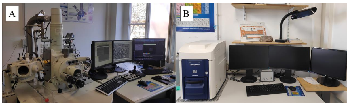
Figure 17 Jeol 640 Scan Electron microscope (A), and TM4000 Plus Hitachi Tabletop Scan Electron Microscope.
