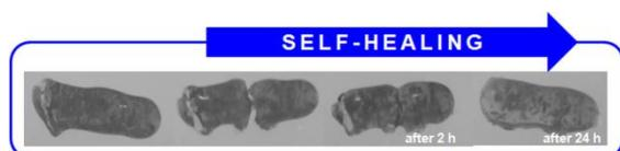
**Fig. 5** Macroscopic self-healing experiments of a cut specimen of **crosslinked 4b** after CuAAC at 20 °C
