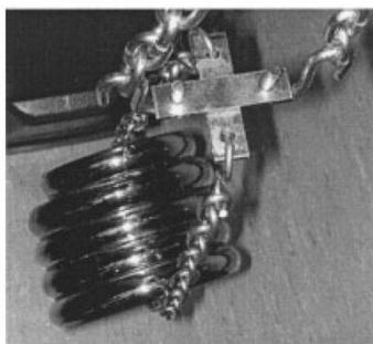
**Figure 3:** Determination of the load bearing capacity of adhesives *via* peel test with crossed copper plates. Figure reprinted from reference<sup>[11r]</sup> with permission from John Wiley and Sons (Copyright 2004).
