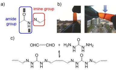
**Figure 12**: a) Chemical structure of the acylhydrazone functionality combining a reversible imine bond and a hydrogen bonding amide group, b) left – virgin polymer film; right – cut polymer film which was healed within the overlapping domain (see arrow), c) equilibrium between a bis-aldehyde and a carbohydrazide and the formed acylhydrazone. Figure reprinted and adopted from reference<sup>[166]</sup> with permission from John Wiley and Sons (Copyright 2014).
