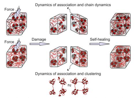
**Figure 6:** Self-healing of a supramolecular rubber after a force-induced damage event *via* re-association of (self-)complementary hydrogen bonding interactions (upper bank) or *via* cluster formation (bottom bank). Figure reprinted and adopted from reference<sup>[48a]</sup> with permission from John Wiley and Sons (Copyright 2013).
