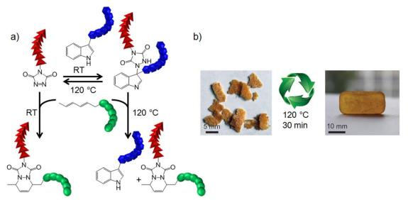
**Figure 11:** a) Overview of TAD based click reactions between TAD and indoles as well as between TAD and dienes. Concept applied to low molecular weight compounds and polymers. b) Image of a crosslinked PU sample, which was healed at 120 °C for 30 minutes. Figure reprinted and adopted from reference<sup>[162]</sup> with permission from the Nature Publishing Group (Copyright 2014).
