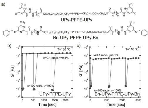
**Figure 9:** a) Structures of bivalent UPy-telechelic PFPE and bivalent Bn-UPy-telechelic PFPE, Multiple deformation-recovery cycles of b) bivalent UPy-telechelic PFPE and c) bivalent Bn-UPy-telechelic PFPE. Figure reprinted from reference<sup>[93]</sup> with permission from John Wiley and Sons (Copyright 2013).
