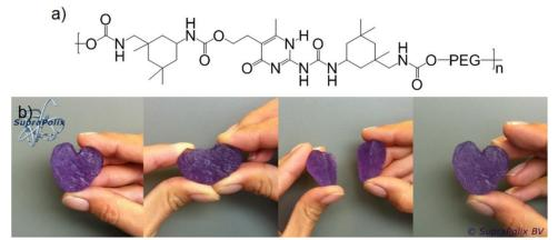
**Figure 8:** a) UPy-functionalized PEG, b) Self-healing of an UPy-functionalized PEG heart (colored by adding a purple dye, 15 wt% in water): initial heart shape was reestablished after pressing cut halves together. Figure reprinted and adopted from reference<sup>[40]</sup> with permission from SupraPolix BV and John Wiley and Sons (Copyright 2012).
