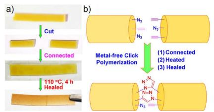
**Figure 4**: a) Self-healing of poly(aroyltriazole) films at 110 °C, b) proposed self-healing mechanism *via* metal-free click polymerization. Figure reprinted from reference<sup>[11ad]</sup> with permission from the Nature Publishing Group (Copyright 2013).
