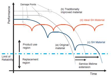
**Figure 1:** Implementation of self-healing principles in engineered materials for service lifetime extension. Figure reprinted from reference<sup>[1d]</sup> with permission from Elsevier Ltd. (Copyright 2014).
