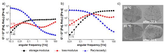
**Fig. 3**: Frequency sweeps of four-arm star thymine-telechelic PIB **3** a) at 20 °C, b) at 40 °C and c) macroscopic self-healing experiments of a cut specimen at 20 °C (upper part) and 40 °C (lower part).
