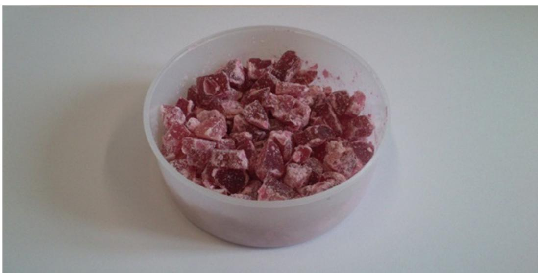
**Fig. S4.** Step D of wax preparation: The crushing of the hardened wax to small fragments.
