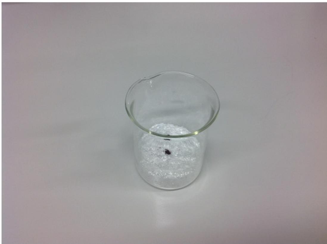
**Fig. S1.** Step A of wax preparation: The weighing of one or multiple crystalline alkanes into a vessel. For a better visualization of the wax, the lipophilic pigment Sudan III (Sigma-Aldrich Chemie GmbH, Steinheim, Germany) was added.
