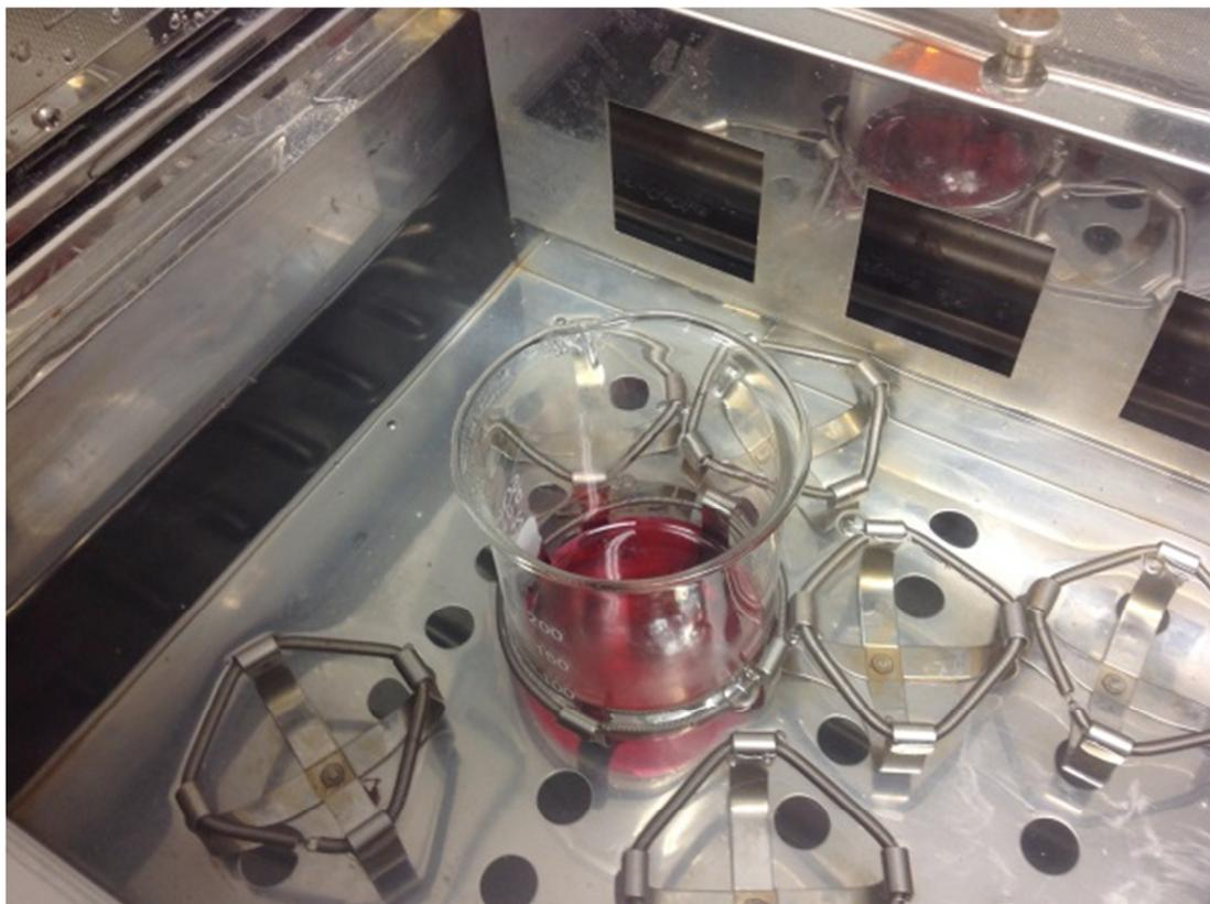
**Fig. S2.** Step B of wax preparation: The melting of the alkane or the mixture of multiple alkanes in a water bath.
