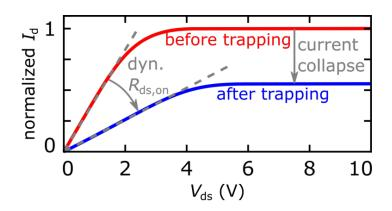
Figure 2.3: Effects of current collapse and dynamic  $R_{ds,on}$  on the drain current with respect to the gate source voltage [KŤ20].
