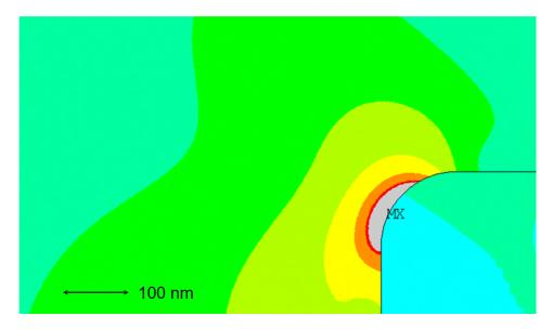
Figure 4.24: Magnification of stress on the gate edge facing the source side with a rounding of the edge.
