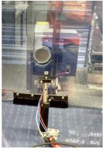
(a) DUT placed in HV housing. In the background the scanning head can be seen.
