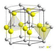
Figure 1.1: GaN Wurtzite structure [08]
