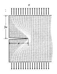
(a) Plate with pre-crack. The roughly triangular stress free area can be seen to both sides of the crack
