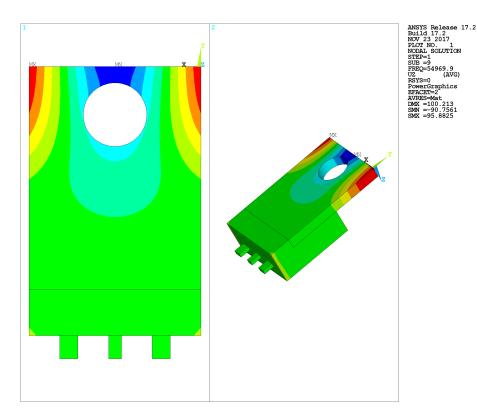
Figure 5.17: Exemplary result of the modal analysis, where the swinging form of the 10<sup>th</sup> eigenmode at a frequency of 54 969.9 Hz is shown. (For the color code note that red marks the maximum positive deflection, while blue marks the minimum deflection)
