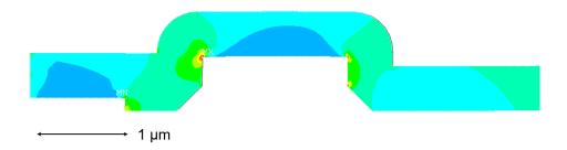
Figure 4.21: Overview of the stress in the ILD layer. It can be seen that the peak first principle stress areas are located on the gate edges. Compared to Figure 4.19 or Figure 4.18 that the geometry of the gate finger has been simplified without affecting the overall result.
