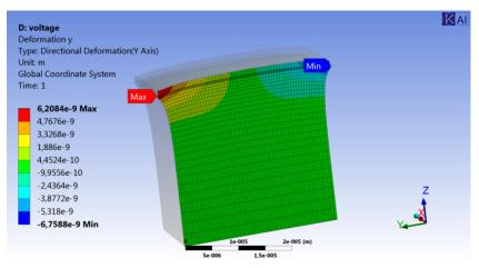
(a) y direction deformation of the stack is subjected to a homogeneous electric field.
