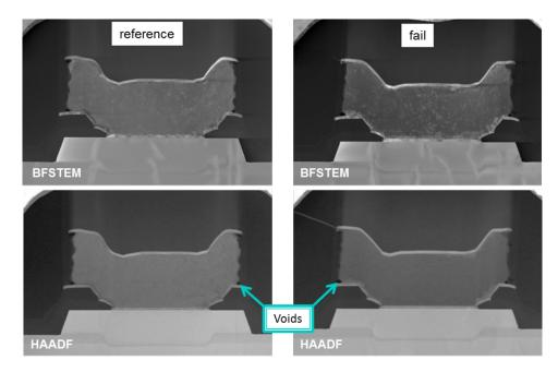
Figure 4.19: STEM and HAADF of gate area. The left picture shows a reference chip, whereas the right one shows a failed region.
