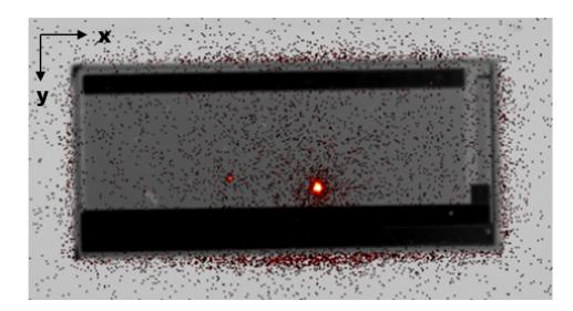
Figure 4.9: Overview of a GaN HEMT. On the top the drain pad can be seen and the source on bottom. The single small pad to the right is the gate pad.(compare with Figure 4.5) PEM performed at the failure analysis labs of Infineon makes it possible to determine the spot of the failure.
