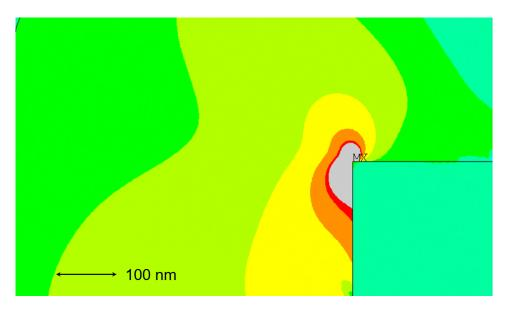
Figure 4.22: Magnification of stress on the gate edge facing the source side.
