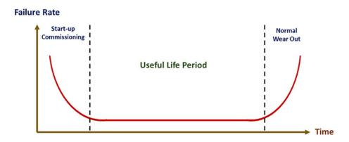
Figure 2.1: A bathtube curve describes the typical failure rate over time [Liv18].
