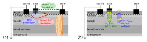
Figure 2.2: Possible break through paths of a GaN HEMT can be seen in figure (a), whereas (b) shows typical trapping sites and their effects [KŤ20].
