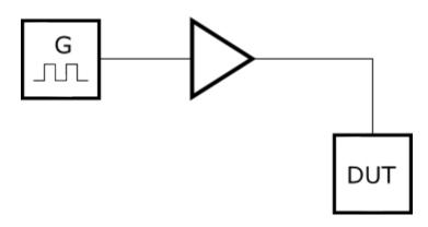
Figure 5.2: Principal circuit diagram of the excited DUT.
