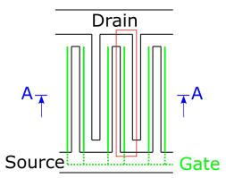
Figure 4.6: Schematic top view of a GaN HEMT, with highlighted drain, source and gate. The red rectangle marks one single cell. The neighbouring single cells show an antiparallel alignment. The gate bus, connecting all the gate fingers is below the big source pad on the bottom.
