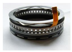
(a) Ultrasonic motor used in an auto focus objective in photography. [Ter08]
