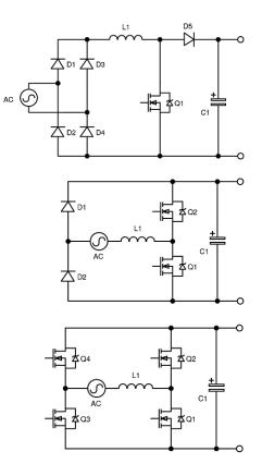
Figure 1.2: Schematics of an ordinary bridge rectifier with a boost converter evolving into a bridgeless totem pole PFC [Li20].
