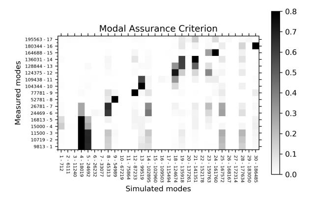
Figure 5.18: MAC matrix comparing all measured eigenmodes with all simulated eigenmodes. Note that each eigenmode is given with its mode number and its frequency.
