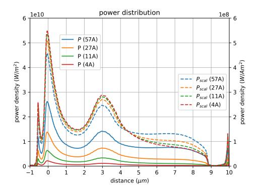
Figure 4.11: Power distributions for different current levels at 400 V. Additionally, also power per ampere is shown on the second y-axis.
