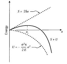
(b) Energy balance between S, the energy needed to form the two new surfaces and U, the energy released by relaxing stress to both sides of the crack
