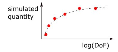
Figure 5.16: (Mesh) convergence of FEM models.
