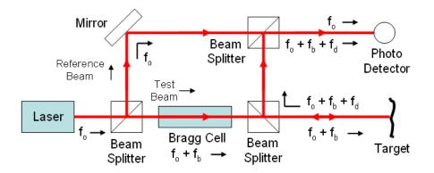
Figure 2.4: Measuring principle of an LSDV [Lad08].
