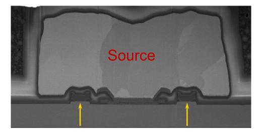
Figure 4.14: SEM picture of a cross section showing the gate source gate area of two single cells. The big source field plate in the middle is covering the gate fingers to the left and right marked with yellow arrows.
