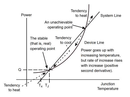
Figure 3.2: Overview of an thermally unstable system. [Sto06]
