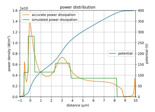
Figure 4.10: Power dissipation and electric potential across the full cell. Distance 0 depicts the gate edge facing the drain side. Additionally the 5 areas and the over all averaged power can be seen in the step function. Note that this is an exemplary graph for 400 V and 27 A. The unit  $W/m^2$  is from the simulation and is meant as Watt per chip area.
