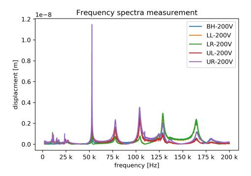
Figure 5.10: Frequency spectra of the five points marked in Figure 5.9. (LL = lower left, LR = lower right, UL = upper left, UR = upper right and BH = body middle) showing seven clear and pronounced resonances (peak voltage used 200 V).
