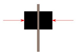
Figure 5.5: Adapted clamping, where the legs of the package are pressed by the jaws of the vise, giving defined mechanical boundary conditions.
