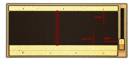
physics. An overview of an actual GaN chip is shown in Figure 4.5, where a single cell is marked in red.
