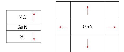
Figure 5.15: Meshing strategy for the test chip. The left figure shows the stack from a side view the right one a top view picture.
