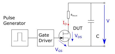
Figure 4.2: Circuit layout of the stress test bench.
