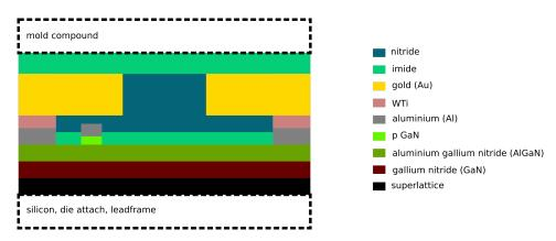
Figure 4.8: Schematic (not in scale) of a single GaN cell and the materials used.
