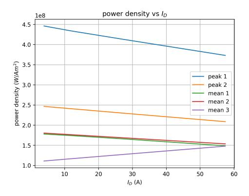
Figure 4.12: Linear regression of the power distribution in W/m<sup>2</sup> for different current levels at  $V_{DS} = 400$  V.
