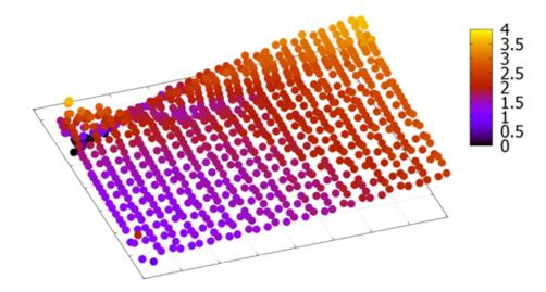
Figure 3.9: Relative difference in percent between the superposition of deformation fields of voltage and temperature separately and the combined approach.
