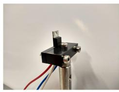
(b) Isometric view on the DUT in the new camping vise.
