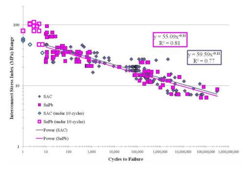
Figure 5.26: Exemplary SN curves of SnPb and SAC solder. [Paq10]
