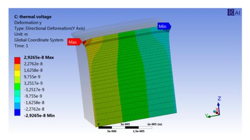
Figure 3.8: y direction deformation of the stack subjected to the temperature change and the voltage at once.
