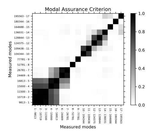
Figure 5.19: MAC matrix comparing all measured eigenmodes with each other.
