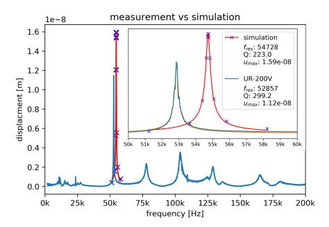
Figure 5.20: Result of the harmonic simulation. Each blue cross is the result of one single simulation. For easier visual inspection the blue crosses are fitted with the red line. The purple line is the measured deformation of the same point. (Orange depicts the fit of the measured result)
