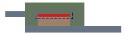
Figure 5.22: Schematics of the cut boundary conditions within the TO-220 assembly.
