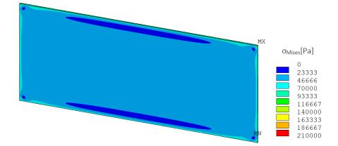
Figure 5.27: Von Mises stress of the die attach layer.
