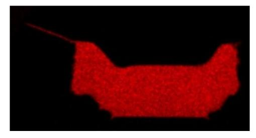
Figure 4.16: Elemental map at the point of protrusion. It can be clearly seen that the crack in the ILD is completely filled with aluminium from the gate finger causing an electric short between gate and source.
