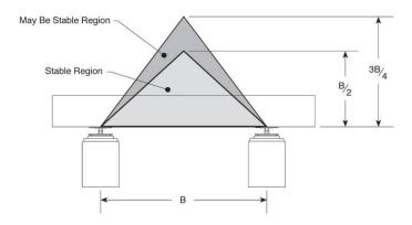
Figure 5.3: Pyramid of stability of the passively damped optical table. [14]
