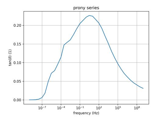
Figure 5.21: Representation of the prony series as loss modulus  $\tan(\delta)$  over frequency.
