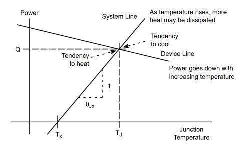
Figure 3.1: Example stability diagram of a thermal system. [Sto06]
