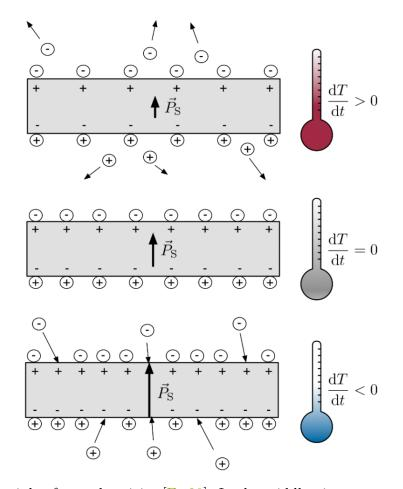
Figure 3.4: Principle of pyroelectricity [Fre20]. In the middle picture a pyroelectric material in thermal equilibrium can be seen. To compensate for the polarisation, surface charges ensure charge balance. If the material is subjected to a temperature change, the polarisation changes due to the changed distance between the positive and the negative charge center. The change in surface charges for charge balance can be measured as current.
