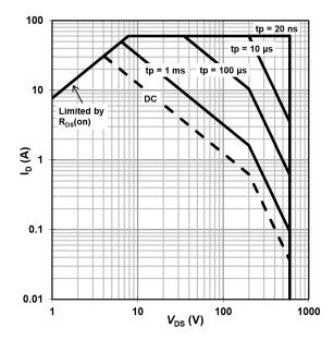
Figure 4.1: Principle SOA diagram of GaN HEMTs [18]. The SOA depends on the time of the pulse. For pulses with a duration of approximately 100 µs, the applied  $V_{DS}$  and  $I_D$  are at least one order of magnitude away from their rated limits.
