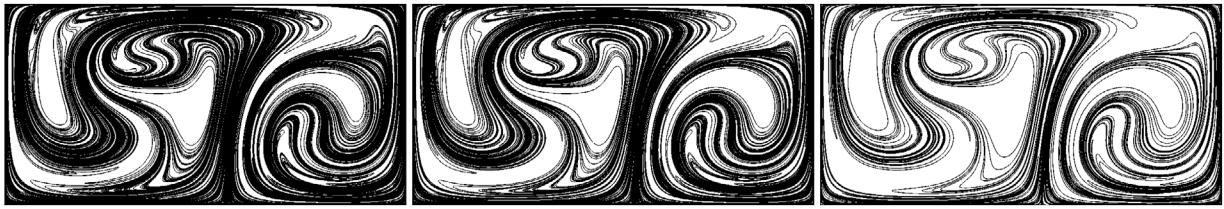
Figure 9: Impact of varying \mu for fixed \tau = 60 . Left: \mu = 1e-2 , arc length = 6943.47. Centre: \mu = 1e-4 , arc length = 3407.08. Right: \mu = 1e-8 , arc length = 837.985.
