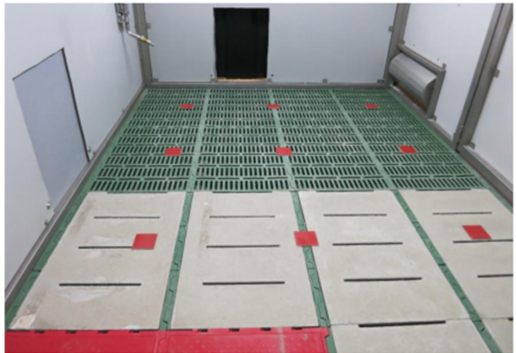
Figure 2. Pen compartment with measuring grid laid out (red metal plates).
