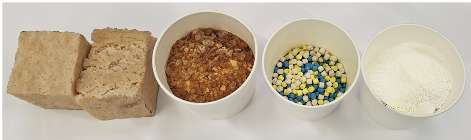
Figure 1.1: Example polymer with various example ingredients. Shown is the polymer, a resin, the curing-system (composed of sulphur, accelerators and retarder) and activators (zinc-oxide and stearic-acid) f.l.t.r.
