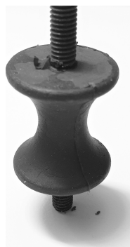
Figure 3.5: Another diabolo-like test piece geometry.
