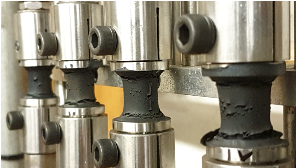
Figure 4.56: NR: Typical multi-crack initiation at the new test piece; shown in the deflected state.
