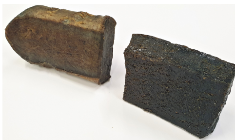
Figure 1.2: Natural rubber and oil extended Styrene-Butadiene rubber.
