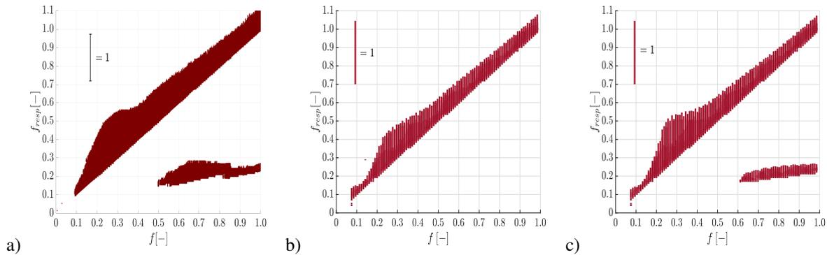
**Fig. 1:** Frequency spectrum of shaft motion: a) measurement, b) simulation with Half-Sommerfeld solution, c) Two-Phase Cavitation
