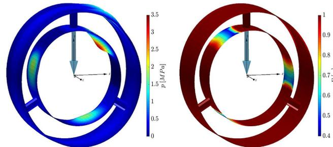
**Fig. 2:** Pressure and lubricant fraction distribution at compressor sided bearing at the beginning of sub-synchronous oscillations  $f = 0.6$
