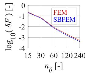
**Fig. 3:** Convergence of the SBFEM and the FEM.
