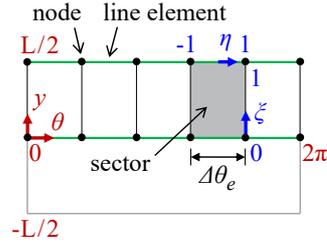
**Fig. 2:** Definition of a superelement on the unwound gap.
