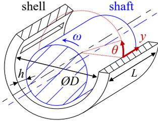
**Fig. 1:** Draft of a hydrodynamic radial journal bearing.
