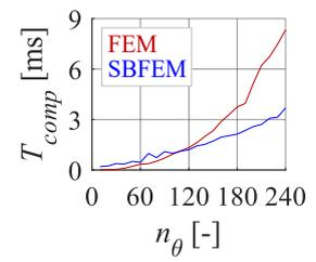
**Fig. 4:** Computational time of the SBFEM and the FEM.
