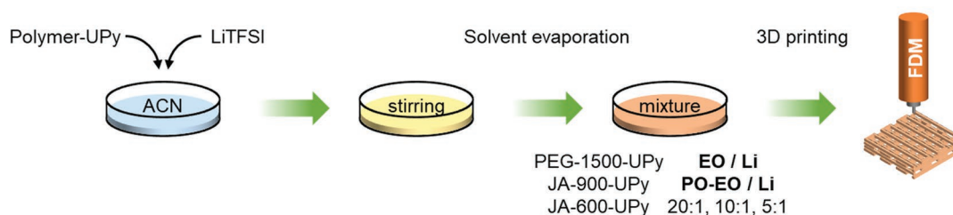
Figure 1. Chemical structure, synthesis, and 3D printing of telechelic, bivalent (2-ureido-4-pyrimidinone) PEG (PEG-1500-UPy), and telechelic, bivalent (2-ureido-4-pyrimidinone) Jeffamine (JA-x00-UPy). Electrolyte mixtures were prepared with LiTFSI for FDM (3D-printing).
