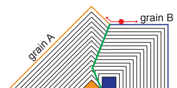
Figure 18: zone T, (top): anisotropy in growth rate leads to V-shaped and faceted columns. This is possible because of allowed intergranular diffusion and grain growth competition; (bottom): magnification of the gray circled region from the top sketch, where an adatom (red) is able to diffuse from grain B (blue line) to grain A (orange line). Both grains grew from differently oriented nuclei (blue and orange) which are however terminated by the same facets, giving A the faster perpendicular growth rate. A grain boundary is formed in the process (green).
