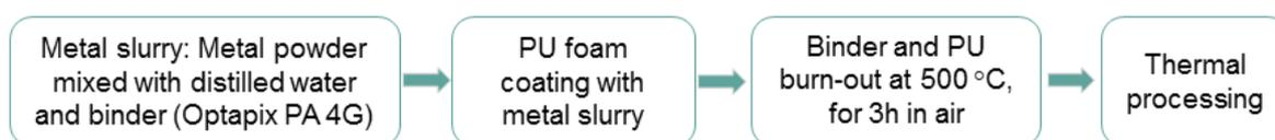
Figure 16 Schematic illustration of RP foams preparation.
