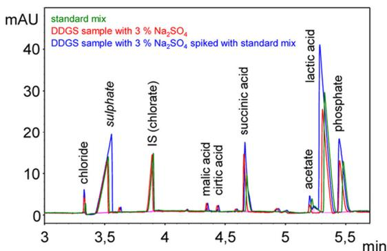
**Figure 4.** Analysis of sulfate in aqueous extracts of DDGS and in pure standard mix (containing different anions and organic acids) by capillary electrophoresis.
