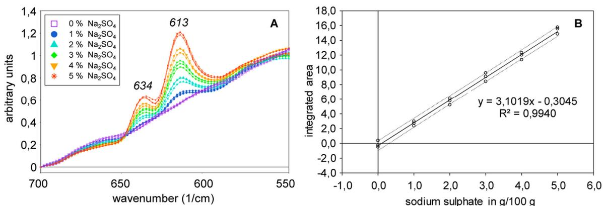
**Figure 2.** FT-IR triplicate spectra of DDGS sample A (SG smoothed, SNV transformed) spiked with different amounts of sulfate (A) and resulting calibration line with confidence intervals drawn by dashed lines (B). Spectra were zeroed to signal at 700  $\text{cm}^{-1}$  in (A) for demonstration purposes (not conducted in actual data processing). Calibration was based on integration of bands between 654 and 586  $\text{cm}^{-1}$ .
