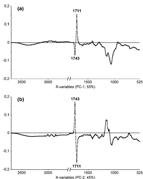
**Figure 6.** PCA loadings plot of FT-IR spectra of oils extracted from DDGS samples for (a) PC-1 and (b) PC-2 indicating the influence of single-wavenumber regions on the variance explained by the respective PC.
