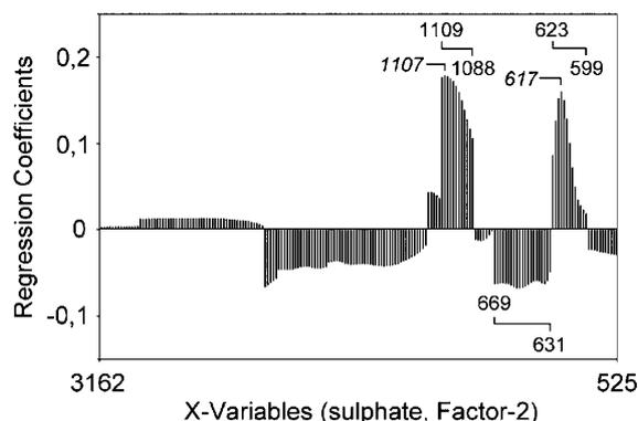
**Figure 6.** Most important spectral variables used for PLS regression and consistency with the fundamental S—O vibrations of the sulfate anion  $\nu_3$  (1105  $\text{cm}^{-1}$ ) and  $\nu_4$  (611  $\text{cm}^{-1}$ ). Scale of X-axis is not continuous.
