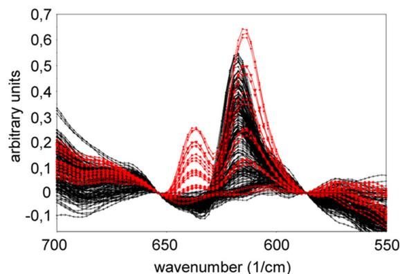
**Figure 3.** Linear baseline correction of preprocessed FT–IR spectra between 654 and 586  $\text{cm}^{-1}$ . Shown are spectra of DDGS sample A, spiked with different amounts of sulfate (red) and spectra of all other DDGS analyzed in the study (black).
