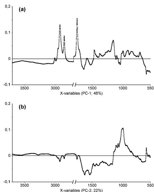
**Figure 4.** PCA loadings plot of FT-IR spectra of solid DDGS samples for (a) PC-1 and (b) PC-2 indicating the influence of single-wavenumber regions on the variance explained by the respective PC.
