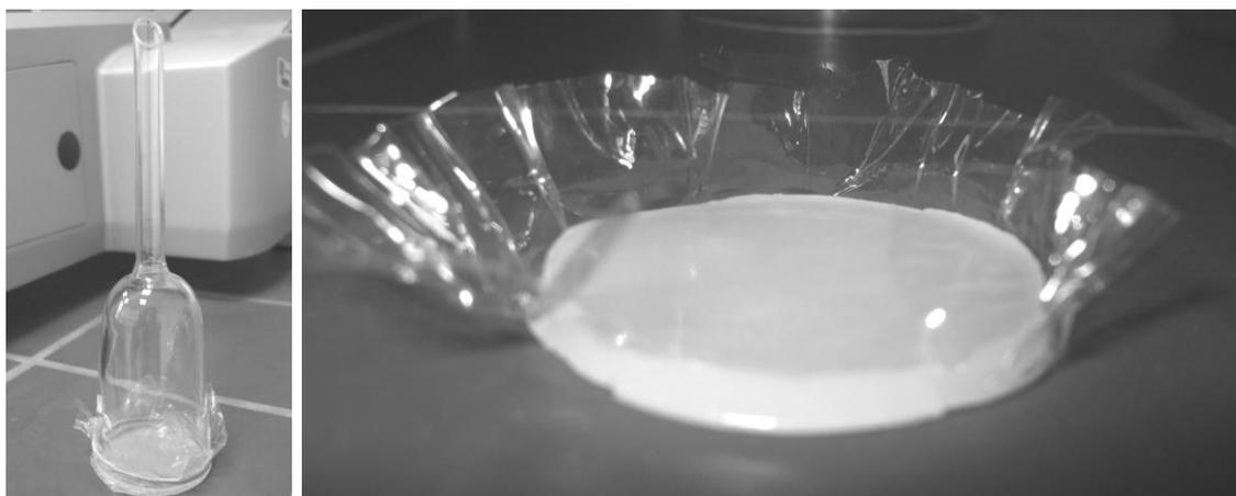
**Figure 6** A self-constructed sample holder consisting of a glass funnel equipped with a dialysis membrane (left), was built to realize the extraction of NMP. The ISFO is located inside of the funnel on the membrane. The solvent NMP leaves the formulation through the membrane into the surrounding PBS resulting in a solidified gel wafer (right).
