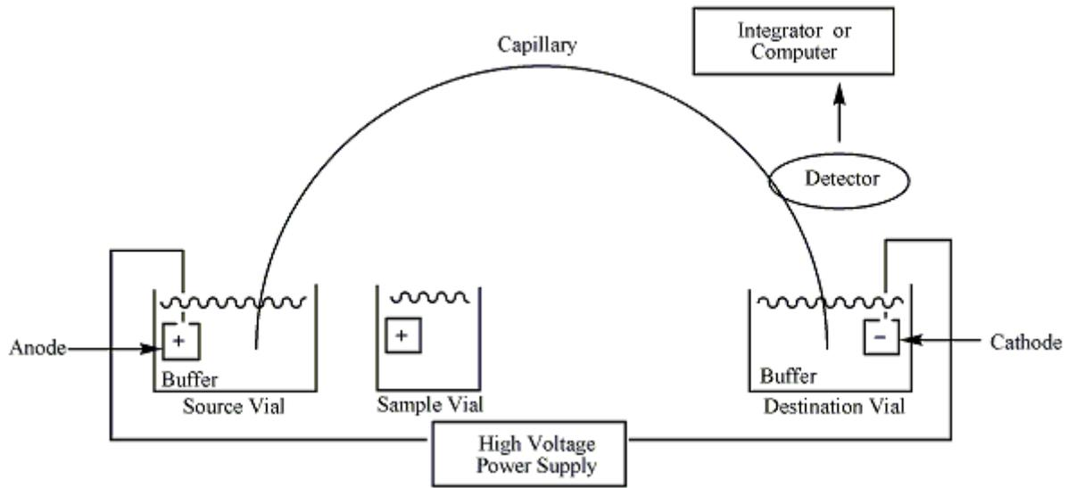
Figure 1 Capillary electrophoresis instrumentation
