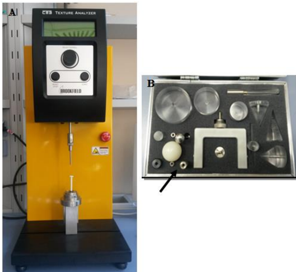
Figure 6. Texture analyzer set-up for injection force measurements. Figure 6A depicts the set-up mounted and Figure 6B shows the tools available for such system, while an arrow indicates the tool used.
