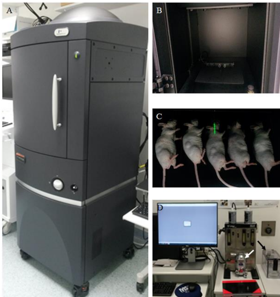
Figure 11. IVIS ® in vivo imaging system (A), inside vision of the plate (B), animals sedated placed on the imaging platform (C) and gas system (D). The white arrow in (D) points to isoflurane container and black arrow points to the induction chamber used to sedate the animals.
