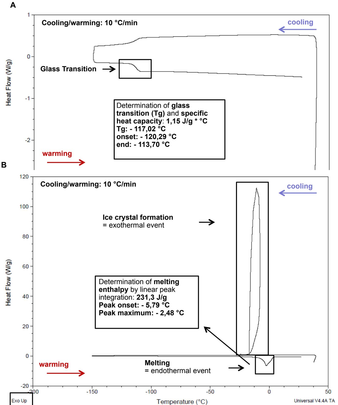
**Figure 7.** Example of DSC thermograms of (A) glass transition events or (B) crystallization and melting event. Calculated specific heat capacity and melting enthalpy is indicated in black rimmed boxes. Speed of cooling and warming: 10 °C/min.
