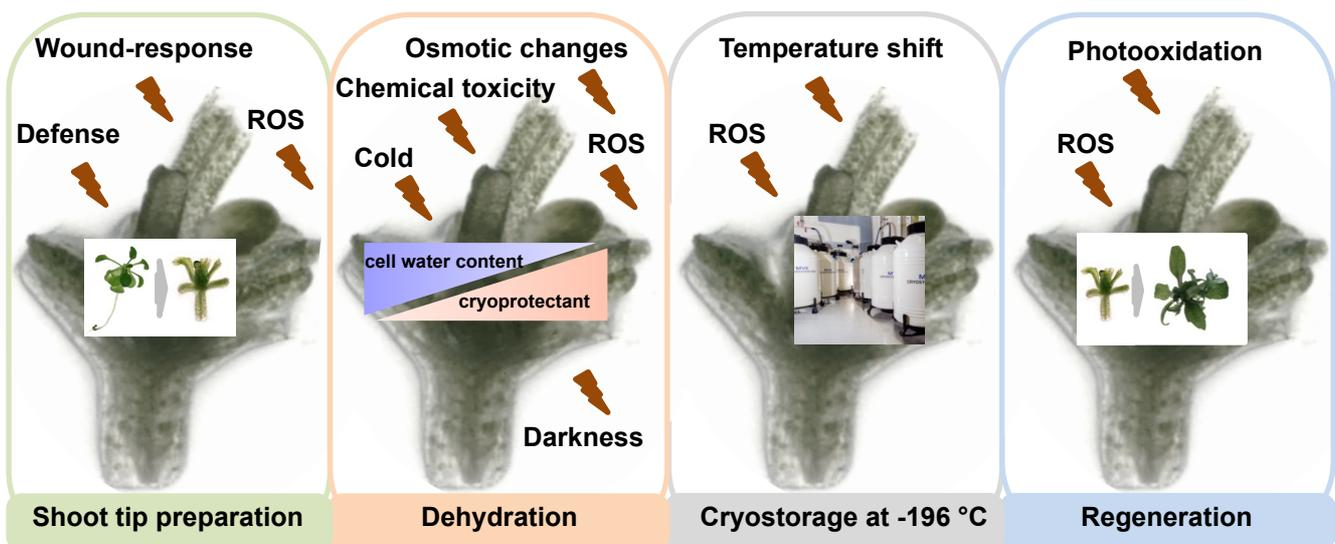
**Figure 5. Cryopreservation – a quantitative trait for different cryostressors.** Schematic overview of putative cryostressors (indicated with red flash) after shoot tip preparation, osmotic dehydration, cryostorage at -196 °C, and during the early phase of regeneration. ROS: reactive oxygen species.
