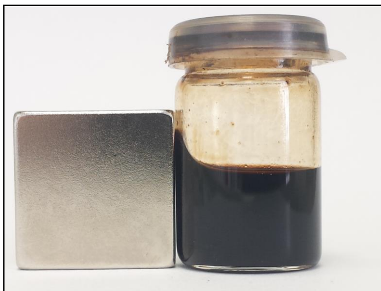
Figure 22: A saturated solution of palmitate capped \text{CoFe}_2\text{O}_4 particles in chloroform next to a permanent magnet. The solution is drawn towards the magnet.
