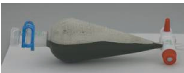
Figure 6-4: Picture of a separation funnel containing sediment and TENAX®.
