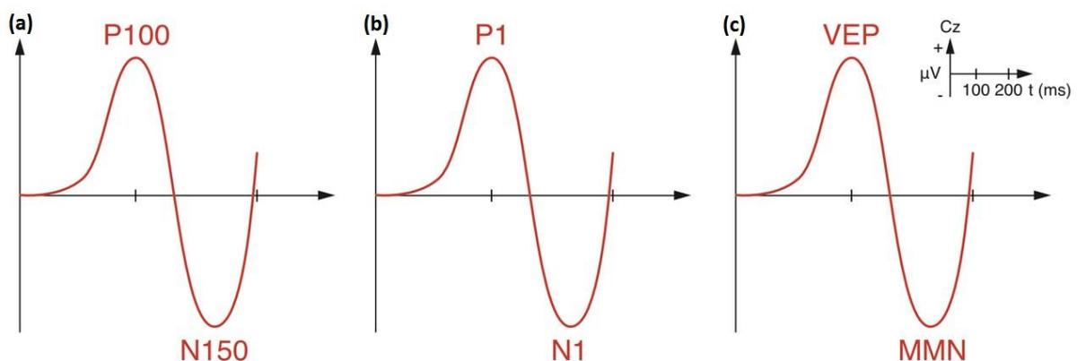
Figure 1.2 Illustration of an ERP signature and labels according to different nomenclatures; (a) = nomenclature 1, (b) = nomenclature 2, (c) = nomenclature 3, VEP = visual evoked potential, MMN = mismatch negativity
