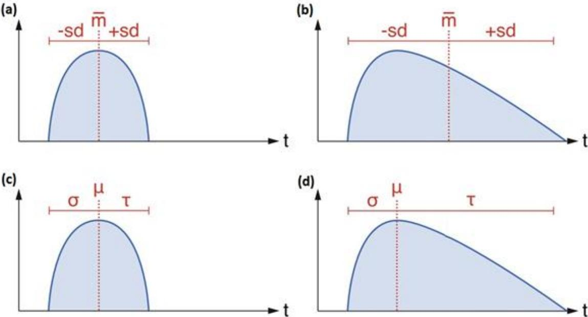
Figure 2.3 Influence of response time distributions on the parameter fit of response time models; (a) and (c) represent the model fit on a normal distribution, (b) and (d) represent the model fit on a non-normal distribution of response times
