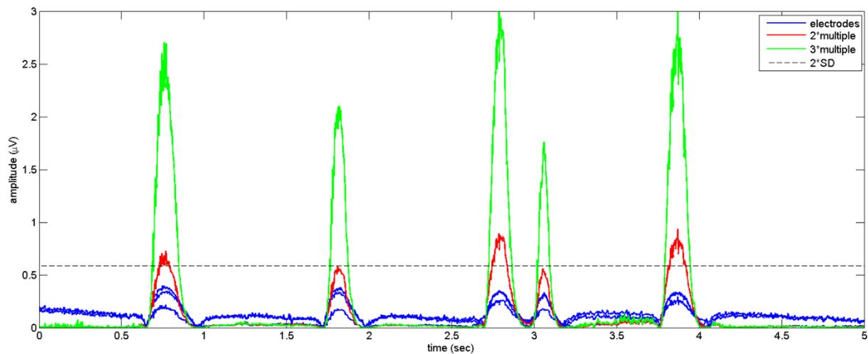
Figure 2.1 The effect of the eye blink detection algorithm; signal of the vertical EOG, Fz1, and Fz2 channels (blue), the product of two channels (red) and the product of all three channels (green). The dotted line represents the detection threshold for the 3\* multiple. Note the emerging difference between eyeblink activity and the non-eyeblink activity.
