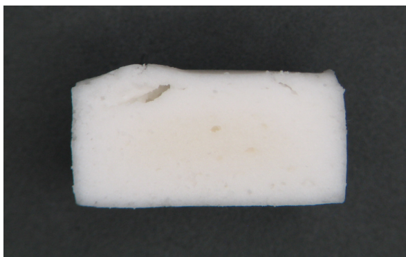
Fig. 6.7 Axial cut tablet with composition H after 9 hours of contact with 0.1 N HCl of 37 °C.
