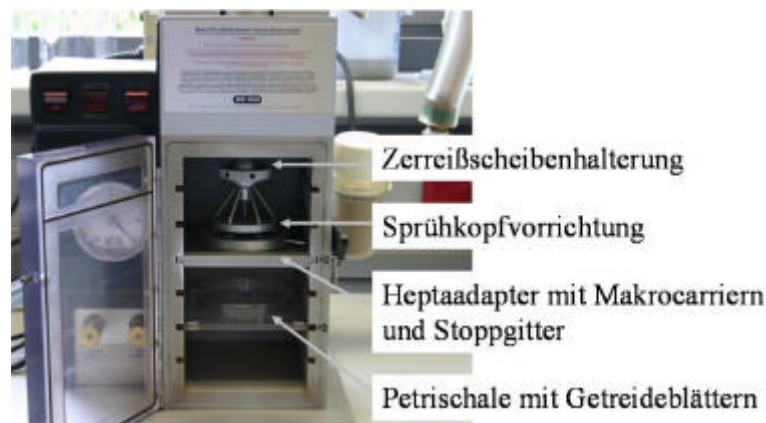
Abb. 2.2: Biolistisches Transformationssystem, Model PDS-1000/He Biolistic Particle Delivery System
