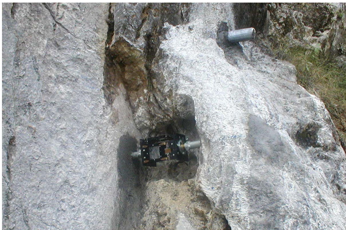
Fig. 4.14: At the monitoring site on the eastern segment of the Shinos fault, the TM71 was installed within an artificial cavity between the footwall and the hanging wall of the fault. The BGX rod was installed behind and above the TM71, also perpendicularly to the fault plane. (Only the protruding end of the BGX rod is visible in the photograph).
