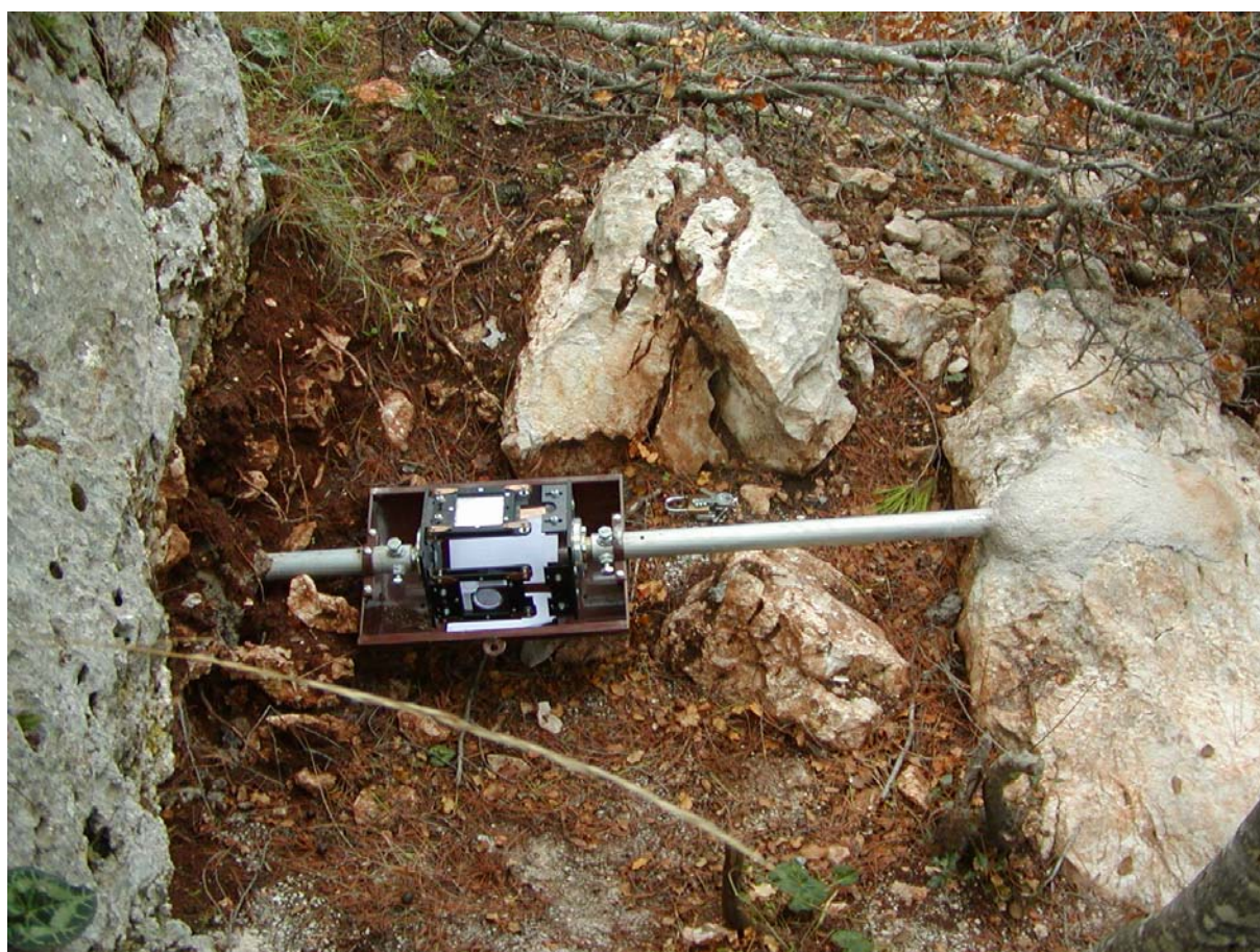
Fig. 4.18: The TM71 was installed between the footwall to the left and a limestone block laying on the hanging wall to the right.
